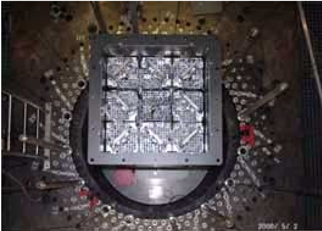
Assembled LWR-PROTEUS Test Zone
