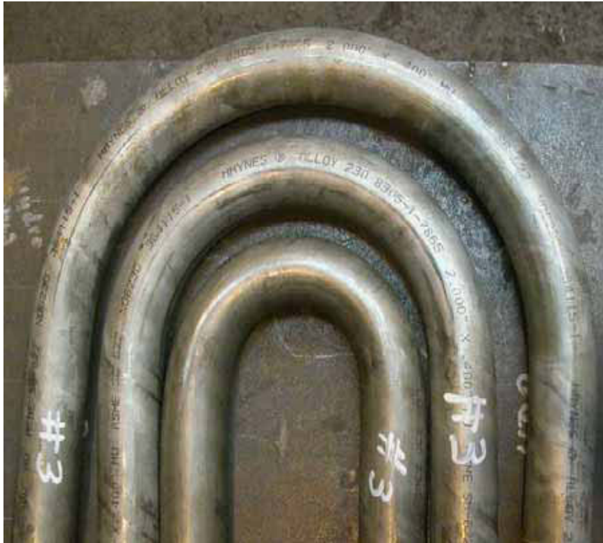
Figure 9. Cold U-bending Trials (Alloy 230 results: R = 3'' , 5'' , 7\text{-}1/2'' (Walt Mohn, B&W).
