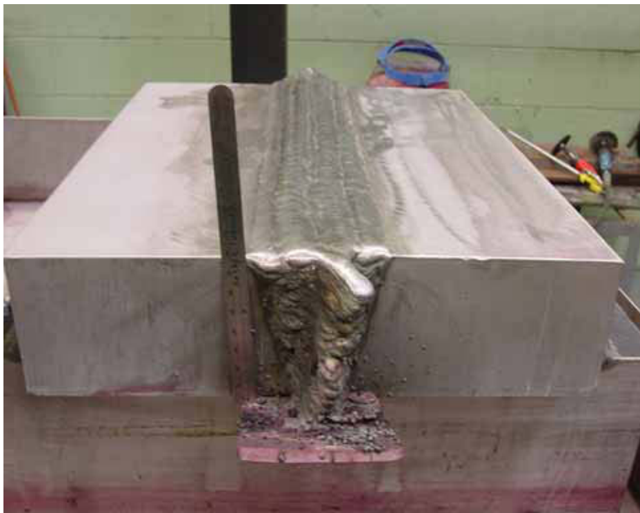
Figure 8. End View of Completed 3" Thick Haynes 230 Alloy Weld (John Sanders, B&W).
