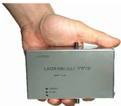
Figure 53.8. Facility monitoring laser particle sensor.
