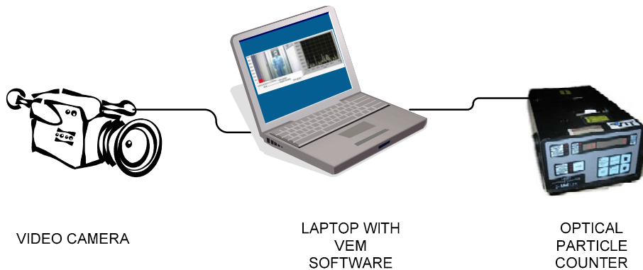
Figure 54.1. Basic configuration of video exposure monitoring system.
