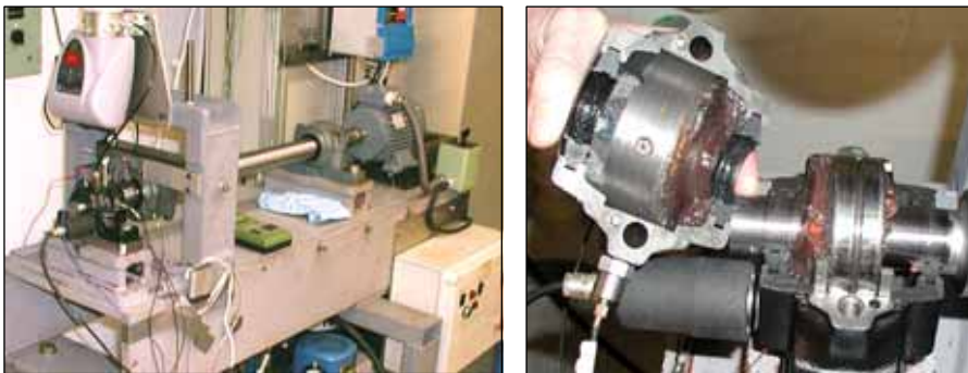
Figure 4. Rolling bearing test equipment with sensors and grease feed mechanism (right). Bearing housing opened after pre-filling (left).
