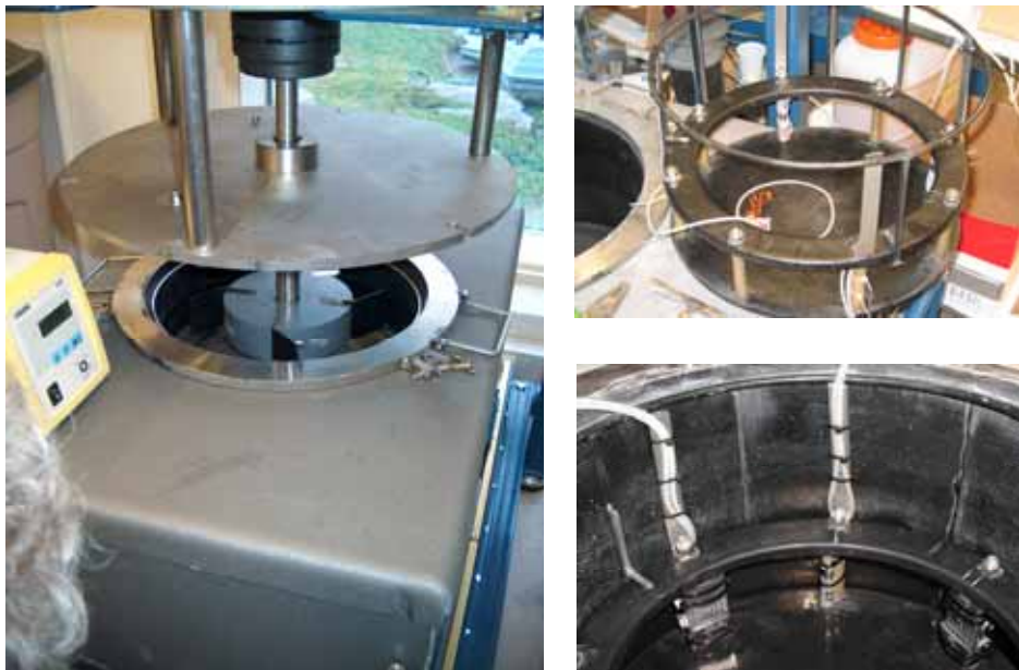
Figure 3. Erosion test equipment consisting of a test chamber and a rotor in the middle. The samples are held near the test chamber walls in a sample holder.
