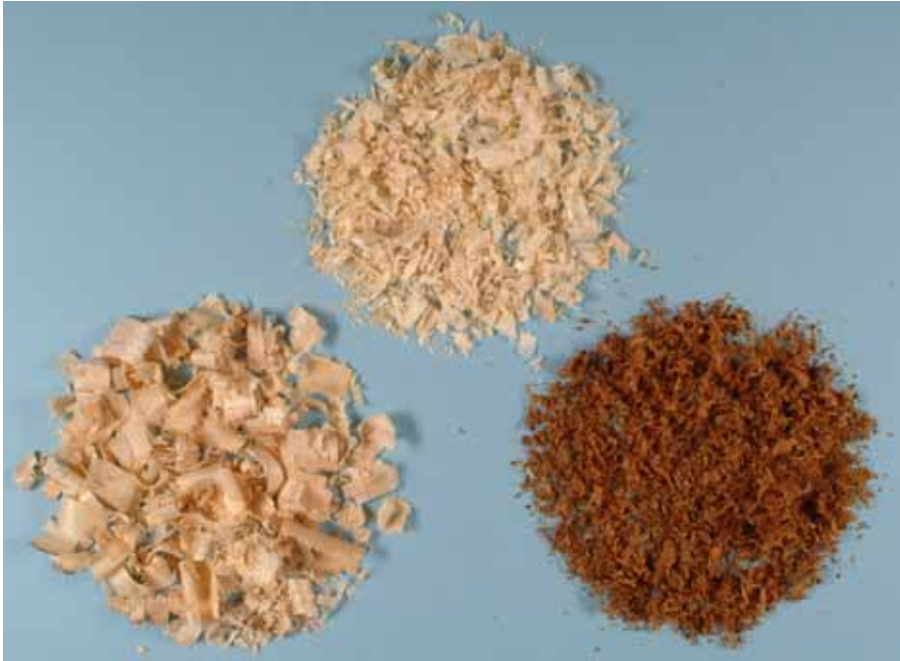
Figure 1. The wooden raw materials used in the WPCs. Above: conifer chips (50% pine and 50% spruce), left: birch chips, right: heat treated pine chips.
