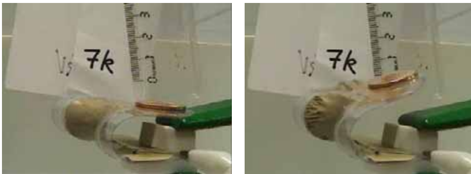
Figure 5. The bending soft frame actuator as a lifter at rest (on left) and at maximum excitation (on right).
