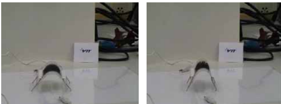
Figure 6. The bending soft frame actuator as a walker in opened step (on left) and in closed step phase (on right).
