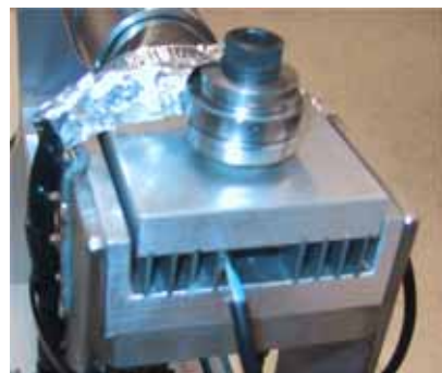
Figure 3. The SMA rib actuator. The bolt force sensor is located at the top.
