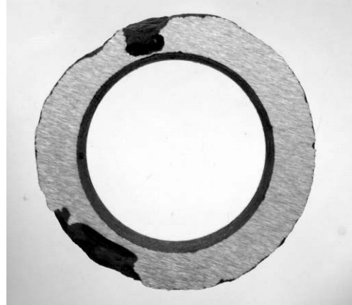
Figure 15. Visible corrosion from external surface.
