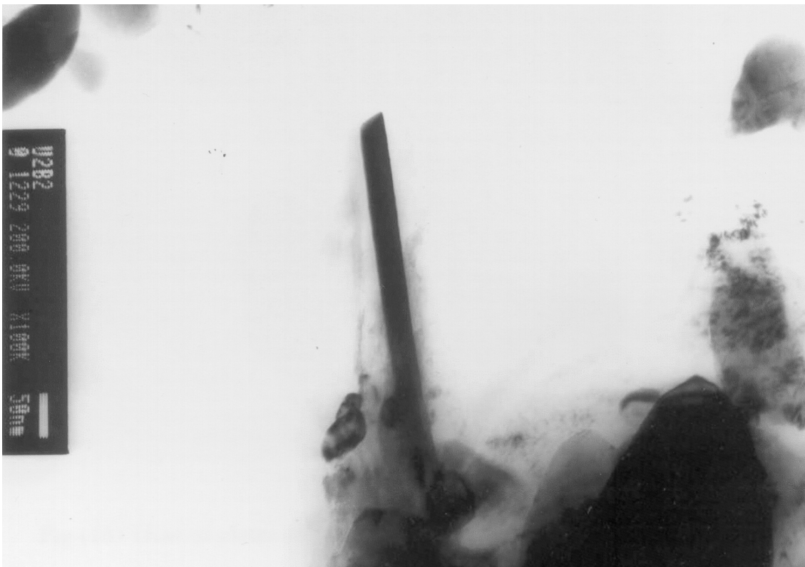
Figure 4. Example of an AlN needle (0.5 \mu\text{m} long) taken from Ref. [5].
