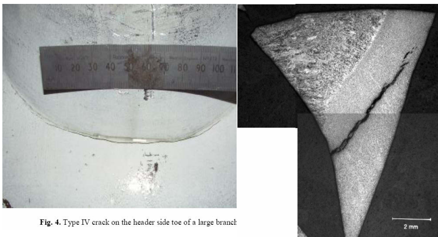
Figure 8. Examples of type IV cracking observed in header welds (15).
