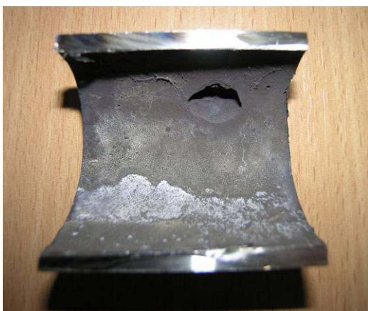
Figure 10. Corrosive pit on upper half of the coil tube.
