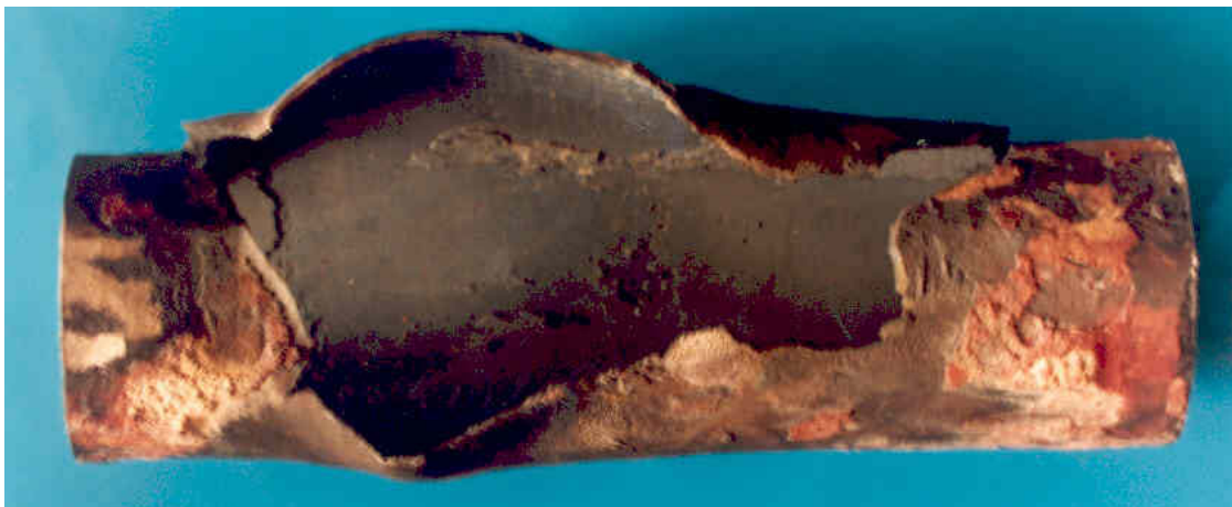
Figure 12. Failures with great deformation.
