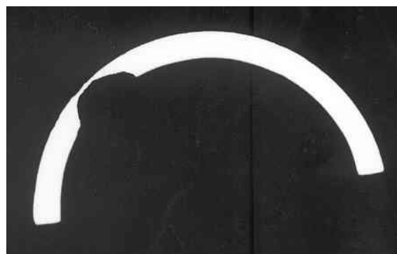
Figure 11. Visible significant wall tube thickness loss.
