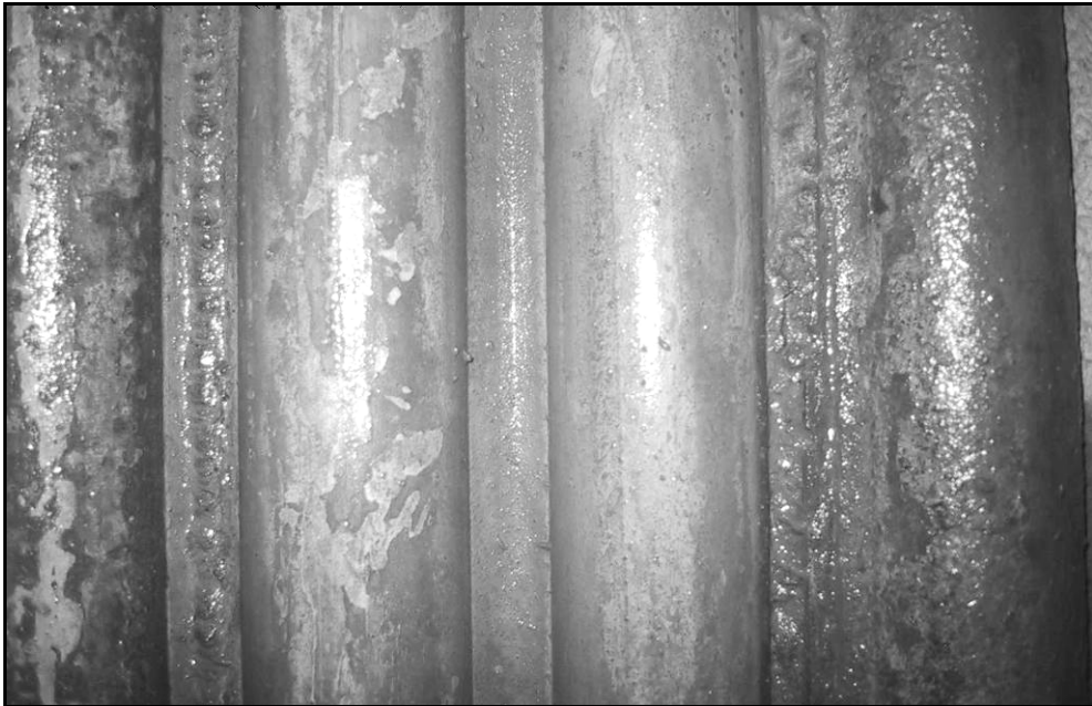
Figure 9. Photograph of the waterwall tubes coated with HybridMD (two central tubes) after exposure during 8000 h, after washing of deposits.
