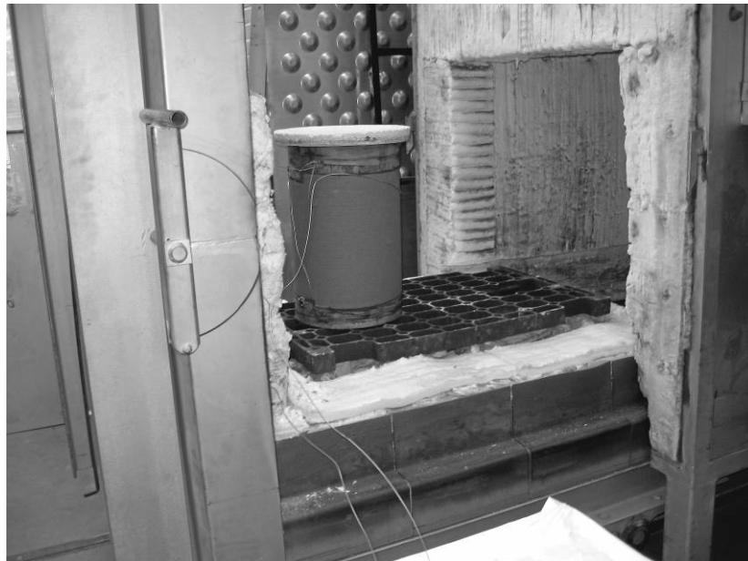
Figure 9. The test object with the embedded fibre is ready for elevated temperature tests in a bogie hearth furnace. The fibre pigtails protected by small stainless steel tubes are seen in the lower part of the picture.
