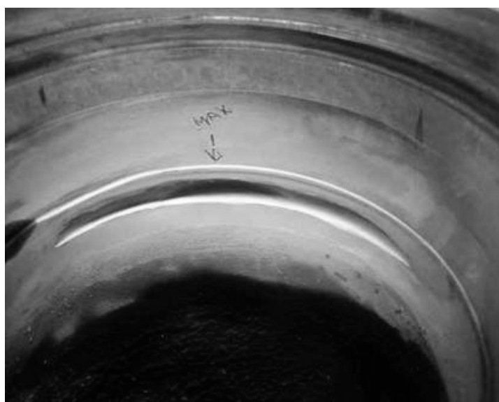
Figure 7. Opening of the crack on the inside surface of the nozzle.
