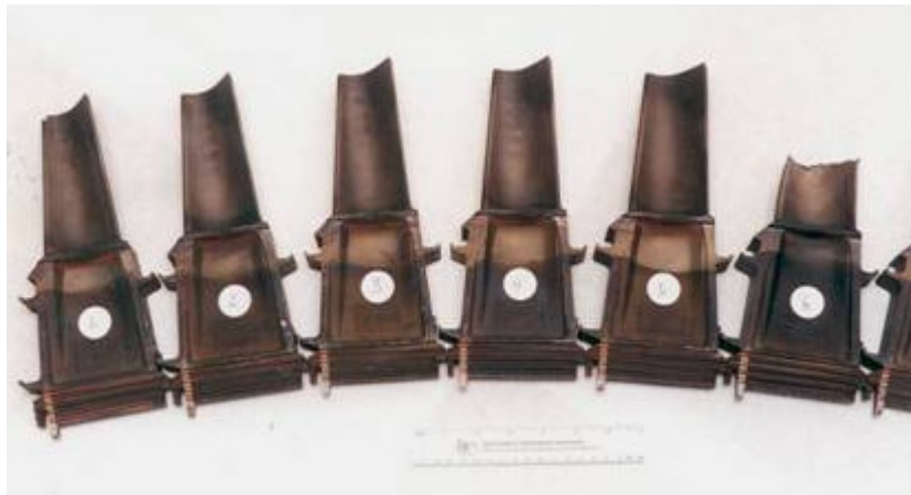
Figure 10. Typical condition of as-received blades.
