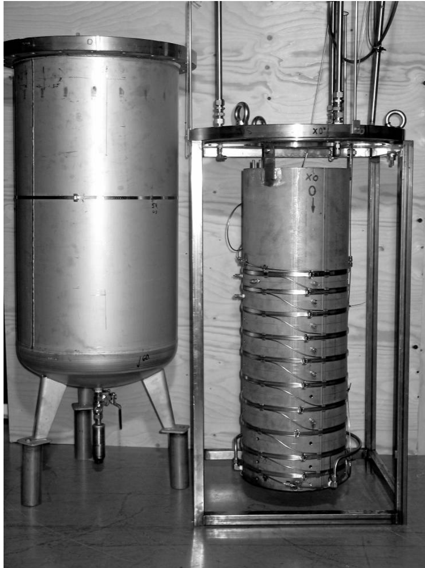
Figure 12. The STYX vessels. The inner vessel is shown to the right with ten zones of fibre (in a stainless steel tube of diameter 3 mm), five turns in each, wound on its outer surface. For the measurements the inner vessel was inserted into the pressure vessel shown to the left. The inner vessel contained sand, heating elements and 48 thermocouples.
