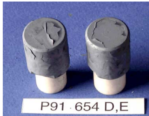
Figure 12. Uncoated P91 samples.
