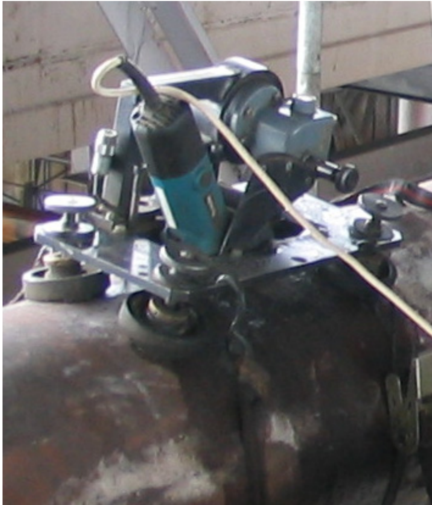
Figure 3. Device MSM-1 for sampling from external surface of power plant components.
