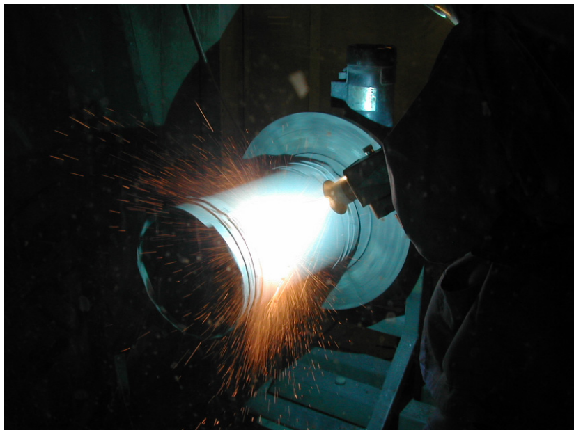
Figure 5. The thermal spray process. About 33.5 m of fibre was embedded in an about 300 \mu\text{m} thick layer of Ni20%Cr coating. The lead-in and lead-out fibres in small stainless steel tubes to the left and to the right are protected by aluminium foils during spraying.
