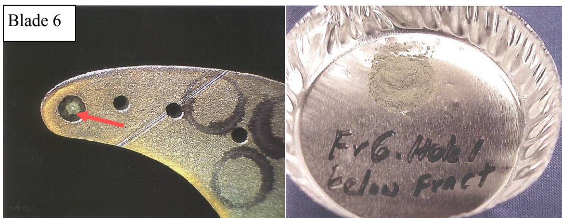
Figure 12. Photographs of deposit in the cooling holes of Blade 6. Arrow on the photographs points to the deposit.
