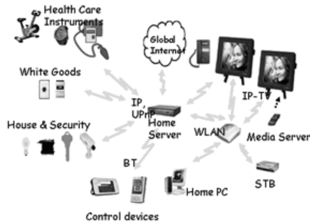
Figure 1. DHS system architecture.
