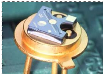
Figure 1. An electrostatically controlled MEMS Micro mirror for the fiber optic variable optical attenuator.
