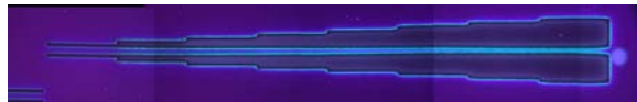
Figure 4. A fluorescence microscope image of InGaN/GaN MQWs grown on the test mask pattern with stepwise increase of mask width.
