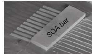
Figure 3. Schematic view of a hybrid integration concept based on thermo compression bonding (left). InP bar with 11 semiconductor optical amplifiers (SOA) flip-chipped on SOI (right).
