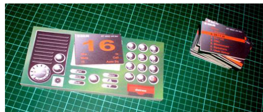
Figure 4. The primitive mock-up made of a print of the front design glued to a piece of cardboard. Changes in the display during interaction were illustrated through exchangeable display cards (the pile to the right in the picture).
