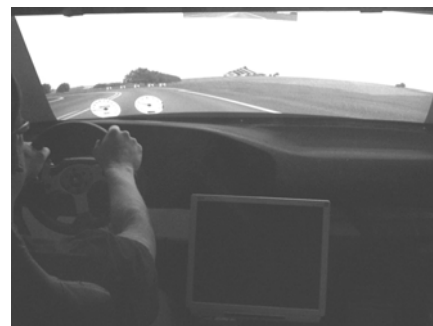
Figure 1. The position of the secondary task display in relation to the driving scene and participant.
