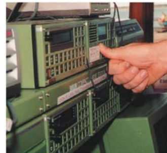
Figure 3. Captain on the supply-ship Skandi Fjord talks about tactile feed-back and shows how he is using existing VHF-equipment.
