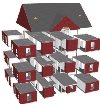
Figure 2. Dormitory exploded view.
