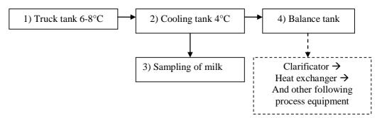
Figure 4. Raw milk flow at the reception point.
