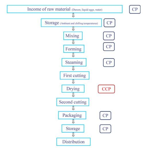
Figure 2. The production process of the egg pasta product is shown in the process flow diagram. CCP's location has been marked on the relevant diagram.
