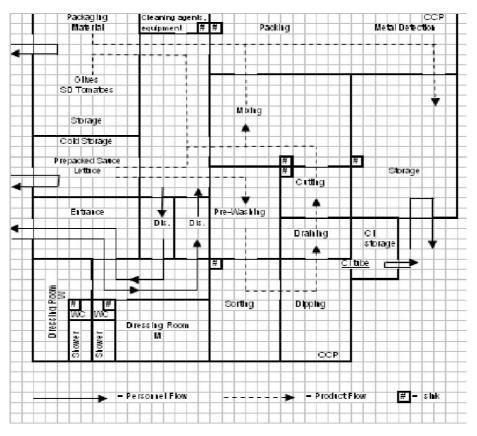
Figure 2. Floor plan for RTE lettuce salad factory.
