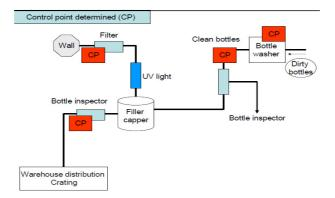
Figure 2. Determination of control points in the water bottling process.
