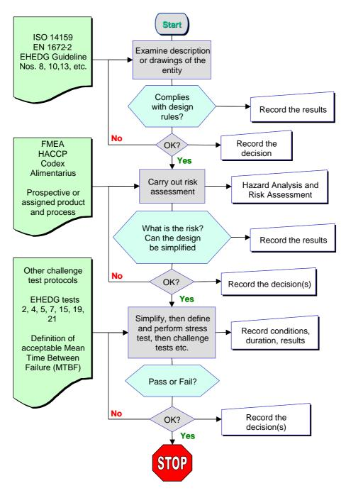
Figure 3. Flow diagram for the integration action 'Validate hygienic performance'.
