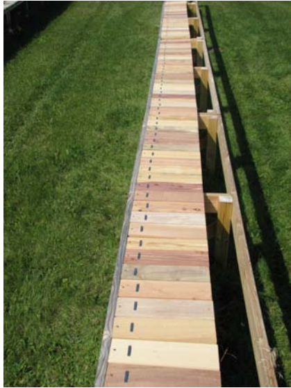
Figure 3. Naturally durable underutilized and invasive wood species in aboveground simulated deck test.
