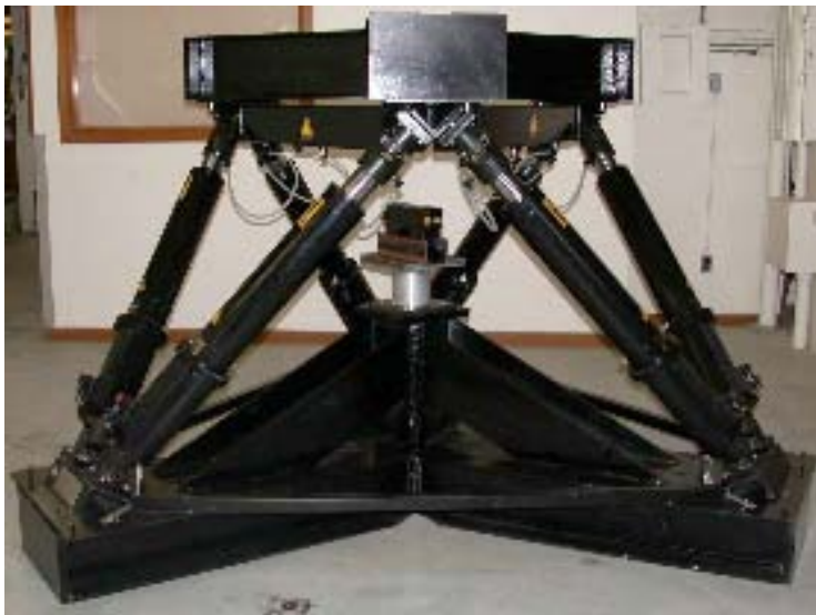
Figure 2. An instantiation at the Forest Products Laboratory of a mechatronic system capable of 6 degree of freedom motion (3 translations and 3 rotations) to test structural materials and systems.
