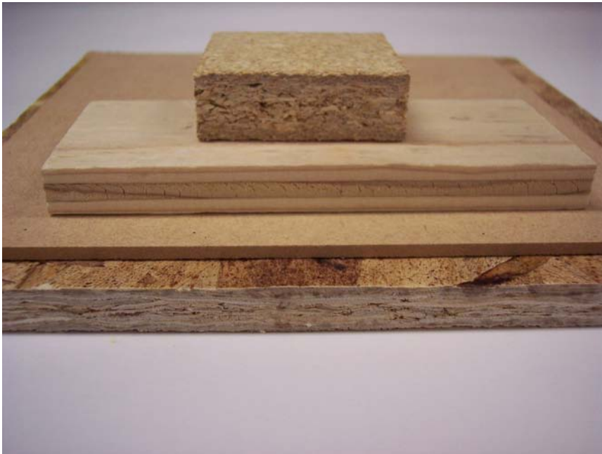
Figure 4. Examples of products made with soy-based adhesives, such as particleboard, plywood, fiberboard, and oriented strandboard (top to bottom).
