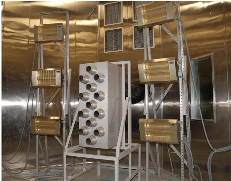
Figure 2. Array of infrared heat lamps and wind nozzle assembly inside the chamber.
