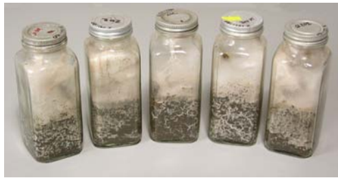
Figure 1. Soil block (or soil-bottle) decay test.
