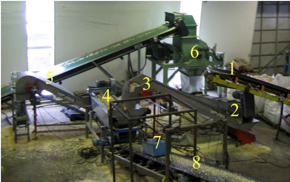
Figure 1. Continuous cleaving and screening process for pulp chips. 1 = feeding of pulp chips, 2 = conveyor of cleaved chips, 3 = feeding pulp chips and cleaved chips on screen, 4 = Pocket Roll screen, 5 = conveyor of oversize chips, 6 = knife mill, 7 = magnet, 8 = conveyor of accepted pin chips
