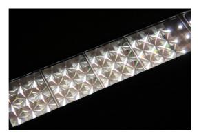
Figure 1. Nano- and micro-structured LED lens matrix for general lighting.
