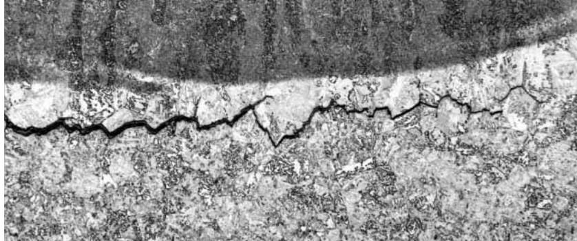
Figure 6. The end section of the crack of specimen CT5 close to the fusion line.
