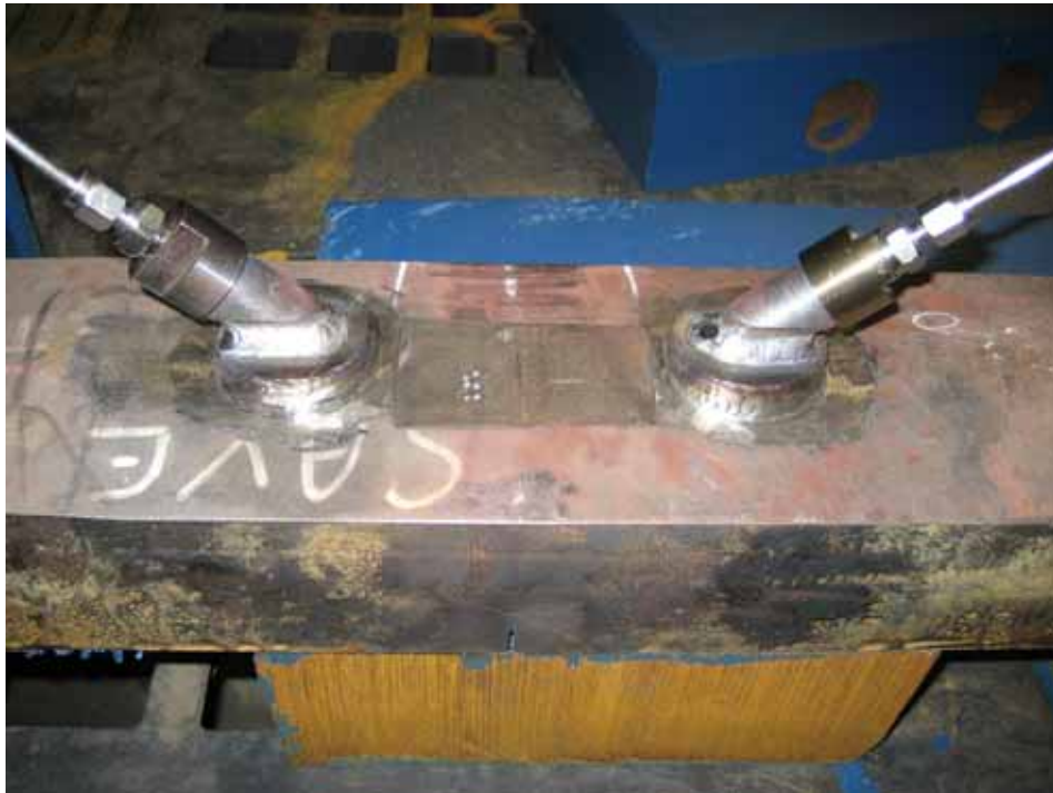
Figure 3. High temperature probes welded onto specimen in TOFD arrangement.
