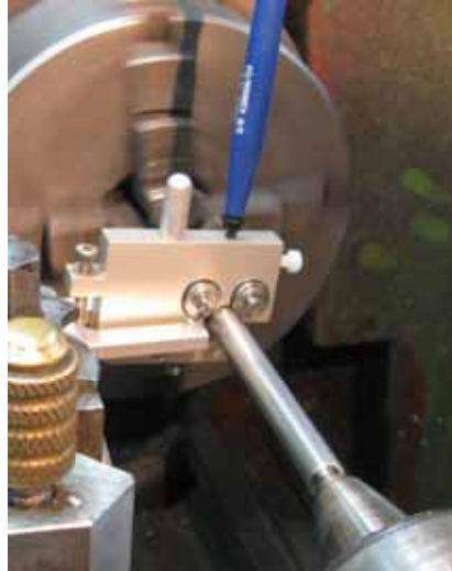
Figure 11. An eddy current measuring setup for tubular sample.
