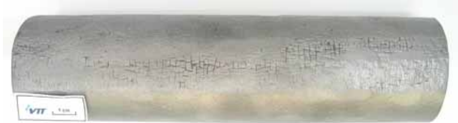
Figure 4. Reheater tube sample (surface oxide removed), with indications of hot corrosion and thermal fatigue.
