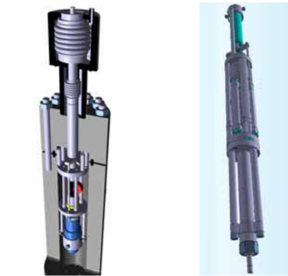
Figure 10. Double bellows SCW (left) and MELODIE (right) testing devices.
