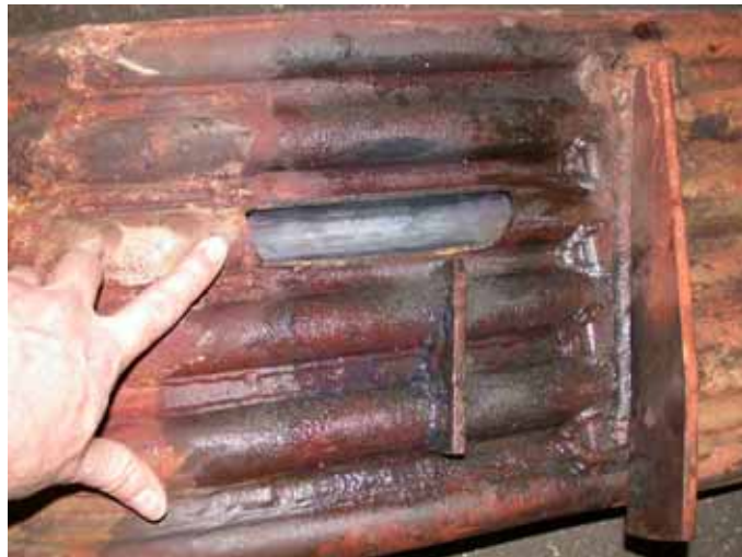
Figure 1. The 2005 tube-burst, showing window blow-out failure.
