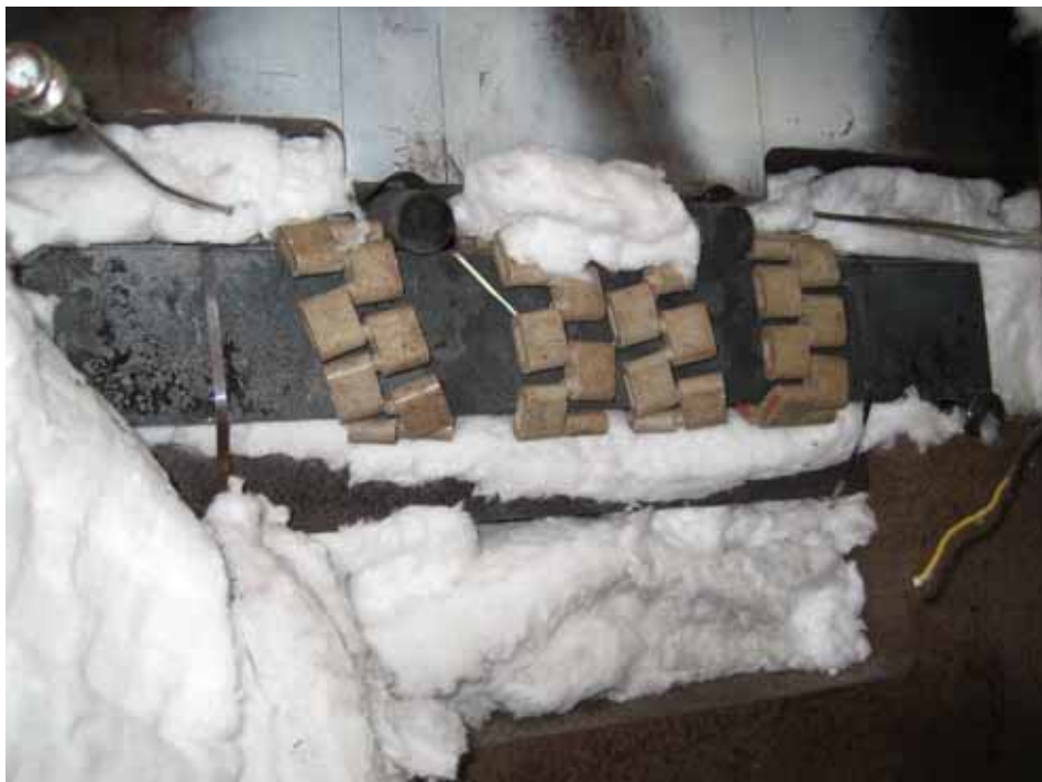
Figure 4. Specimen in 4-point bend rig at completion of test with insulation partly removed to show heating element arrangement.
