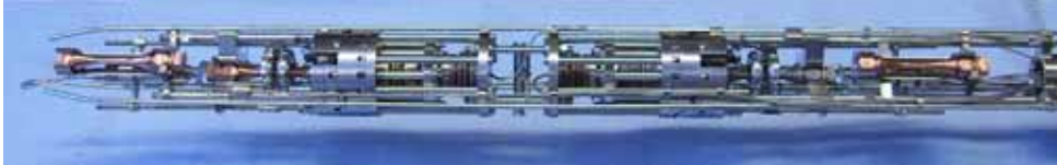
Figure 6. HIPS probe for in-pile fatigue testing
