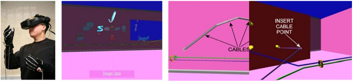
Figure 1. VR Apparatus & Cable Harness Design Functionality.
