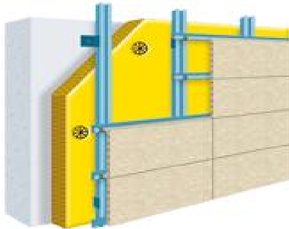
Figure 4. Structure of a ventilated façade. (Vetisol ATLAS)
