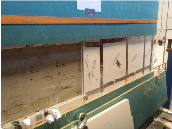
Figure 2. Concept B1 by VAHANEN, vacuum insulated test wall.
