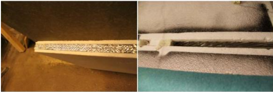
Figure 7. Intact and broken vacuum insulation panels.
