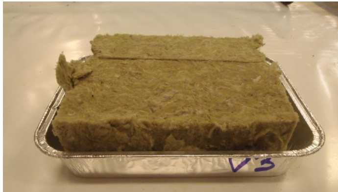
Figure 18. Insulation sample from the test wall. Samples were dried in an oven to determine moisture content as weight percent.
