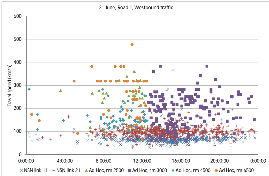
Figure 9. Individual travel speeds calculated from FMD travel time observations on static travel time links and from ad hoc travel times on Road 1, westbound traffic, June 21.
