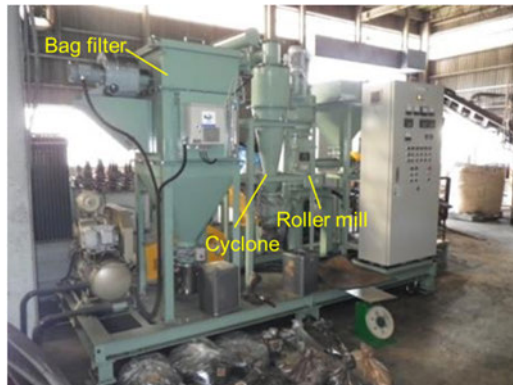
Figure 4. Pilot roller mill for grindability evaluation of torrefied biomass.
