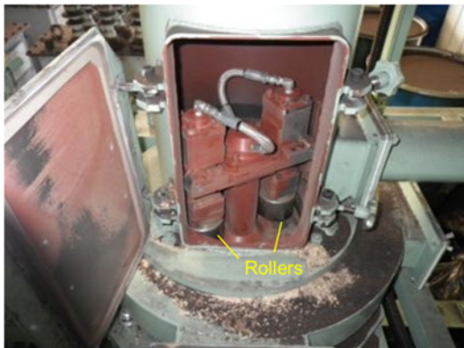
Figure 4. Pilot roller mill for grindability evaluation of torrefied biomass.
