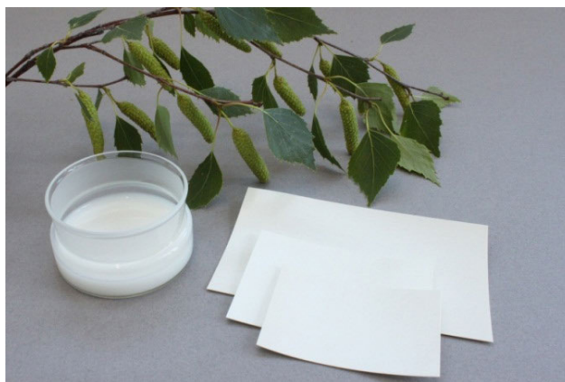
Figure 2. Xylan isolated from bleached birch kraft forms a white dispersion after ultrafiltration or precipitation from the alkaline extract (left). Barrier coating of HPX on pre-coated board (right).
