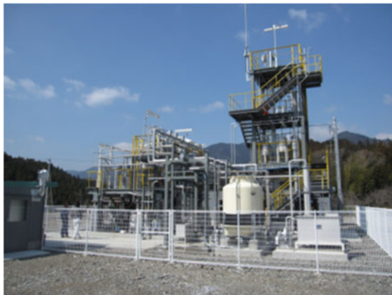
Figure 4. Fourth system plant in Japan for refining lignocellulosics into lignophenols and carbohydrates.
