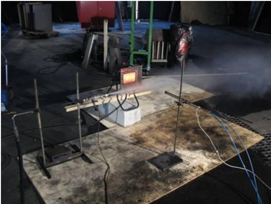
Figure 34. Experimental set-up for measuring the radiation attenuation by water mist micro nozzles.
