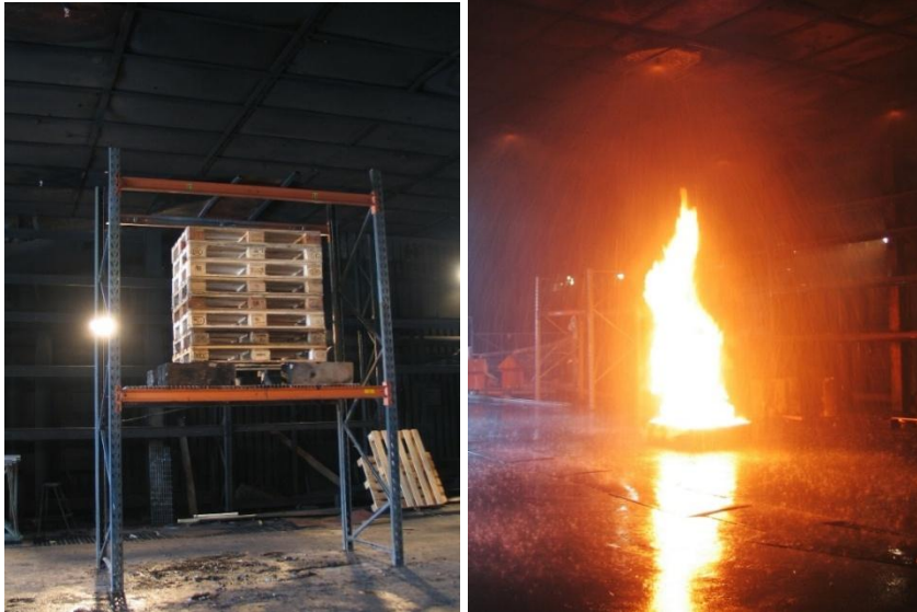
Figure 19. Left: the wooden pallet fire load at 1.5 m elevation. Right: the heptane pan fire between 4 standard spray sprinklers for 4 m ceiling height.
