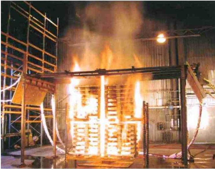
Figure 69. Commodity classification test for idle wooden pallets.
