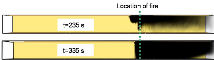
Figure 87. Spreading of smoke for air flow velocity of 2 m/s. Above: moment of suppression system activation. Below: 100 s after water mist system activation.
