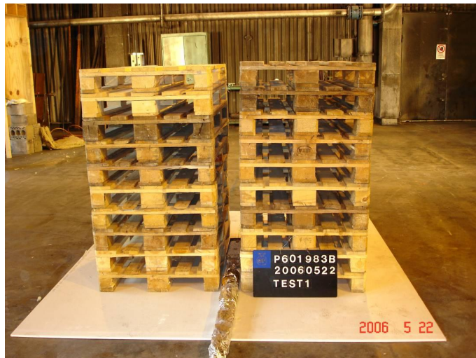
Figure 66. Experimental set-up for a freeburn experiment conducted at SP.
