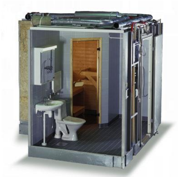
Figure 56. Parma-bathroom elements are delivered on site as completely ready-to-use wet room units, with all the furnishings, fittings and HEPAC equipment installed either from the top or from the side prior to the installation of facades (Parmarine 2012).
