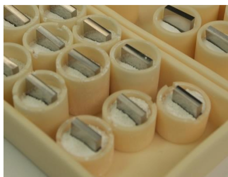
Figure 1. Sample set-up during exposure with deposit, the half of sample covered with deposit.
