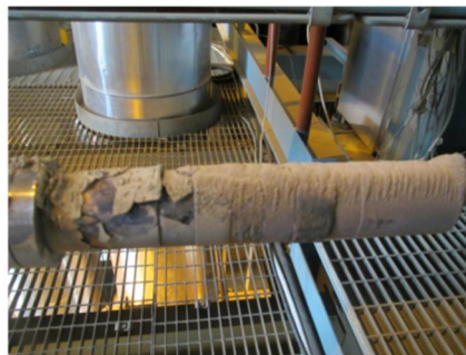
Figure 6. VTT's high temperature probe after 1300 h exposure. On the left material samples at metal temperatures of approximately 550°C and on the right samples around 750°C.
