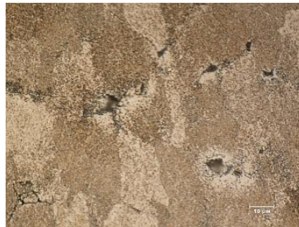
Figure 7. Cavities, mag. 1000x.
