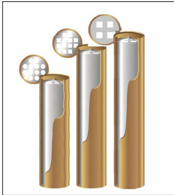
Figure 3. Different types of nodular cast iron inserts for VVER 440, BWR and EPR (from left to right) [1].
