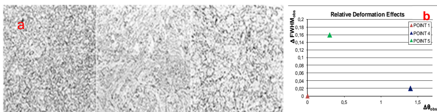
Figure 5. Optical micrographs at magnification of 500X from the metallographic replica of points 4 and 5 of Figure 3 b (a); \Delta FWHM vs. \Delta\theta (b).
