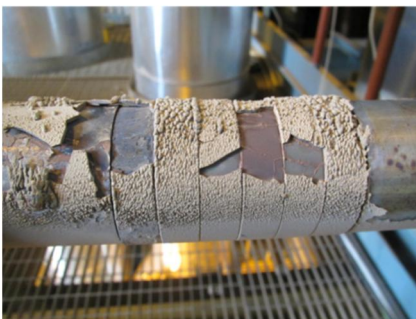
Figure 6. VTT's high temperature probe after 1300 h exposure. On the left material samples at metal temperatures of approximately 550°C and on the right samples around 750°C.
