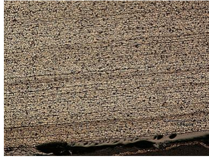
Figure 3. Structure lines, mag. 50x.
