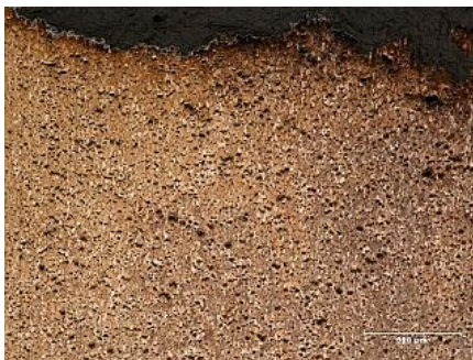
Figure 8. Cavities close to the fracture, mag 50x.
