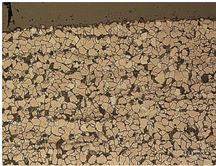
Figure 4. Ferrite – pearlite structure, inner surface, mag. 200x.
