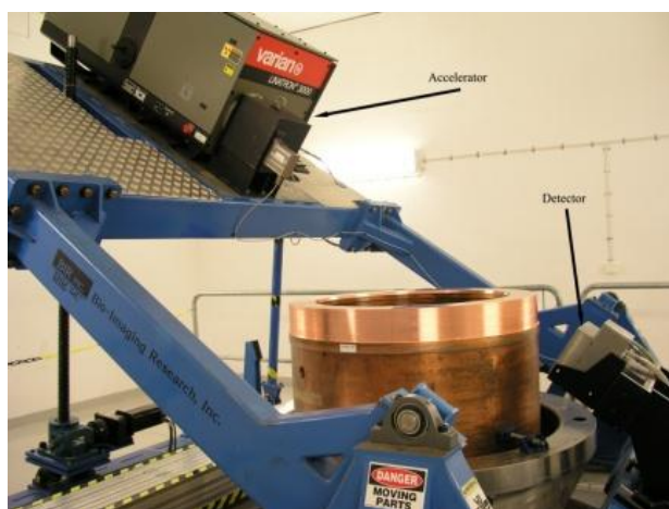
Figure 9. The accelerator and the detector in SKB Oskarshamn site.
