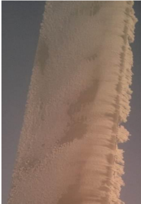
Figure 5. An example photo of an ice accretion.
