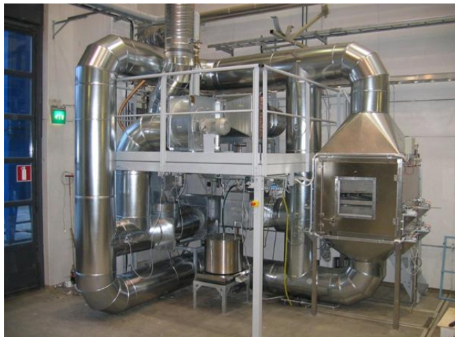
Figure 26. The condensing dryer at VTT used as a climatic testing chamber for the determination of equilibrium moisture content (EMC).
