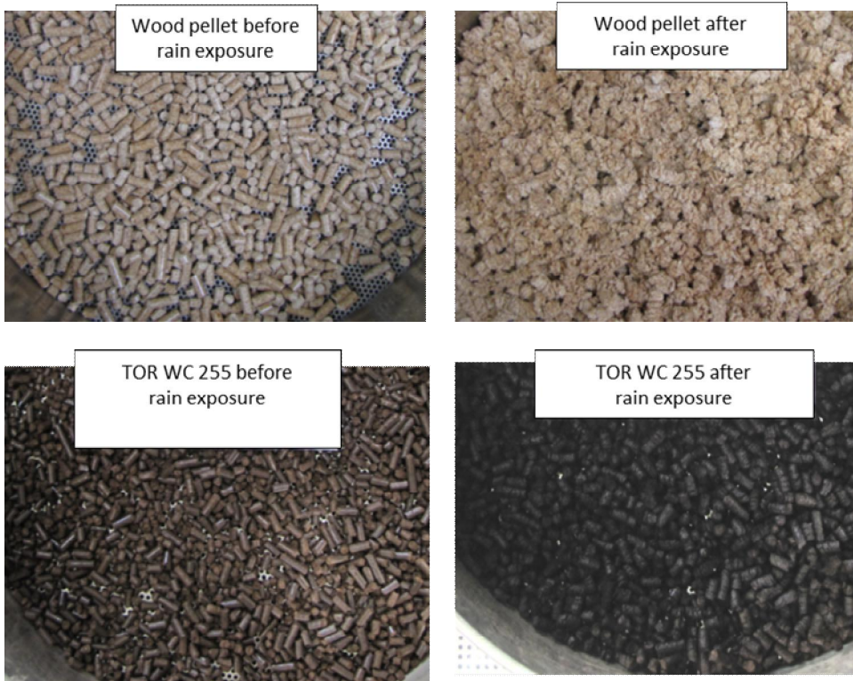
Figure 30. Wood pellets and torrefied wood pellets before and after the rain exposure tests.
