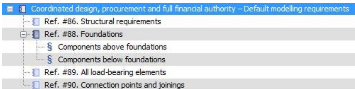
Figure 4.48. Rulesets of Statsbygg BIM Manual in Solibri Model Checker, C.5 Structural Engineering Modelling, Coordinated design, procurement and full financial authority – Default modelling requirements.
