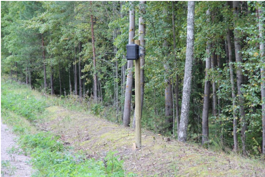
Figure 2. Spot speed measurement device attached to a wooden post.
