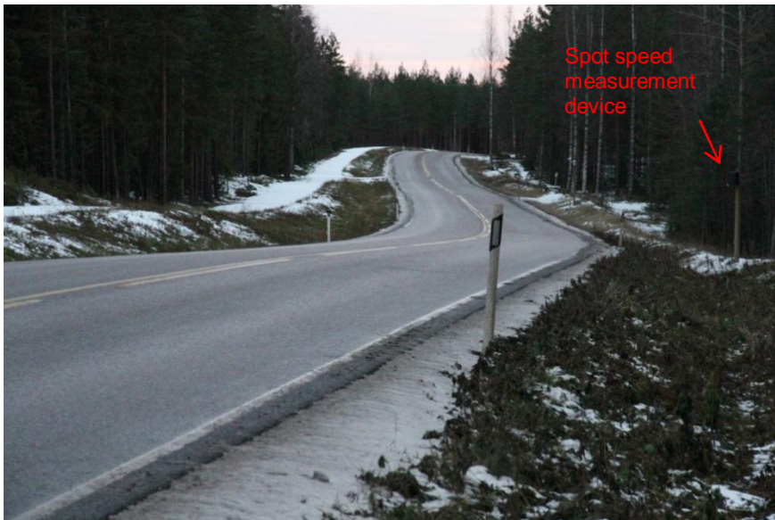
Figure 1. Delineator posts on the test site in early November. The spot speed measurement device is faintly visible on the right of the picture.
