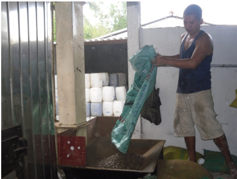
Figure 56. Feeding pellets to the first hopper (Photo by Duc Vu).
