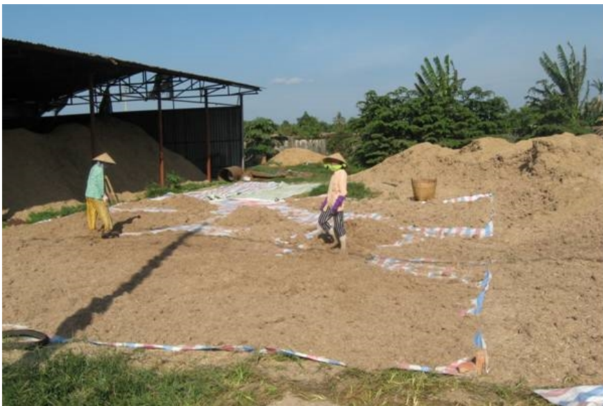
Figure 14. Bagasse is dried on the ground by solar energy for pellet production in Ben Tre sugar mill (Photo by Arvo Leinonen).
