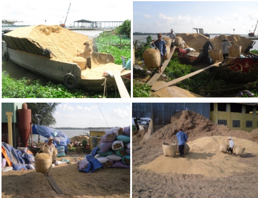
Figure 38. Unloading and manual transfer of rice husks from the boat to the bagasse store areas (Photos by Duc Vu).
