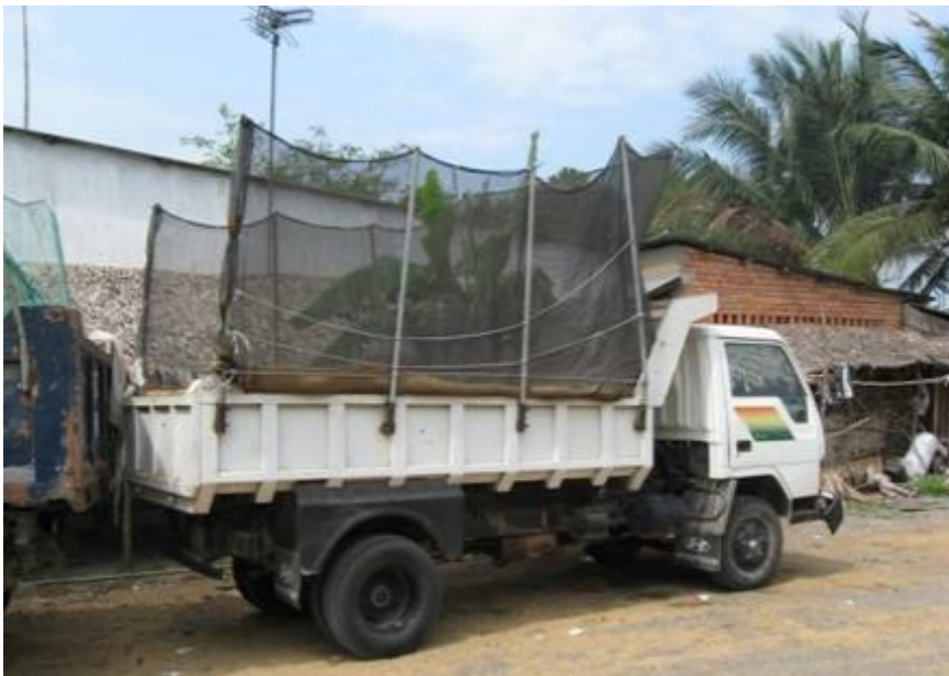
Figure 10. Truck trailer for short transport of rice husk at Dinh Hai power plant (Photo by Arvo Leinonen).
