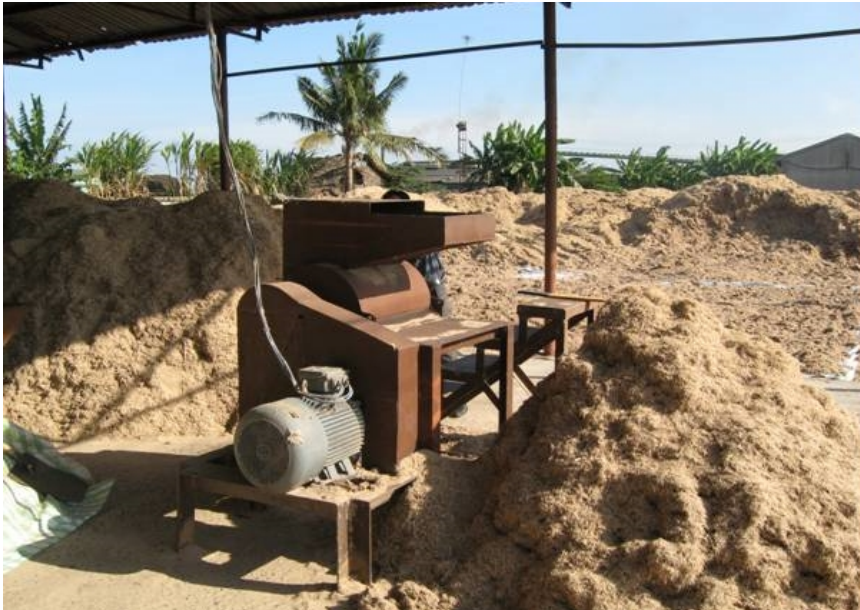
Figure 15. Bagasse is crushed after solar drying with a crusher in Ben Tre sugar mill (Photo by Arvo Leinonen).
