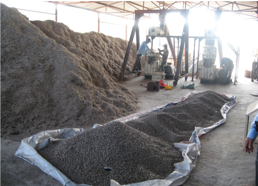
Figure 16. Bagasse is pelletized after drying and crushing in Ben Tre province (Photo by Arvo Leinonen).
