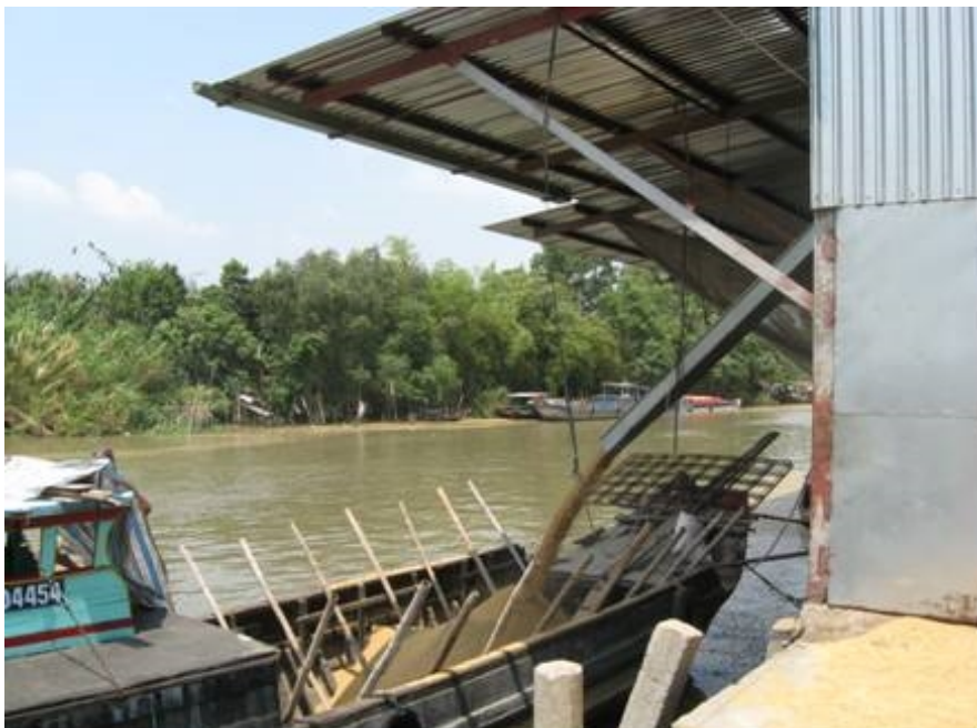
Figure 7. Loading of rice husk into the boat in Nam Nga -rice mill in Tien Giang -province in 2011 (Photo by Arvo Leinonen).
