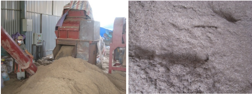
Figure 45. Crushing of bagasse (left) and crushed bagasse (right) (Photos by Duc Vu).
