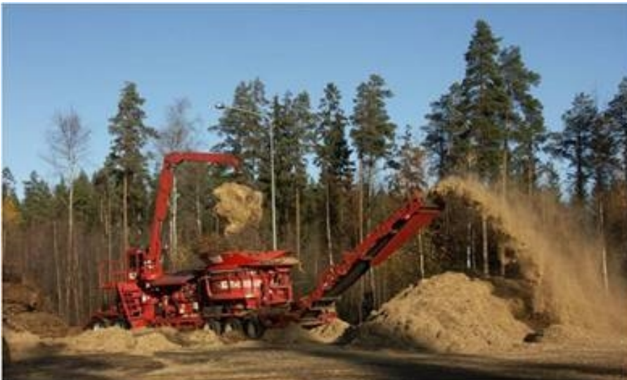
Figure 1/7. Morbark 1200 XL tube grinder. Machine can crush wood and RCG simultaneously. The capacity of the crusher is about 20 tonnes/hour (Rinne et al. 2005).
