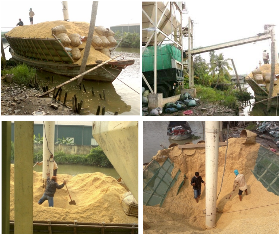
Figure 34. Unloading of rice husk from the boat with the unloading device. The 25 tons boat (up and left) unloading device – suction pipe, horizontal belt conveyor, vertical bucket conveyor and the hopper (up and right), suction pipe (down and left) and suction nozzle (down and right). (Photos by Duc Vu and Arvo Leinonen).
