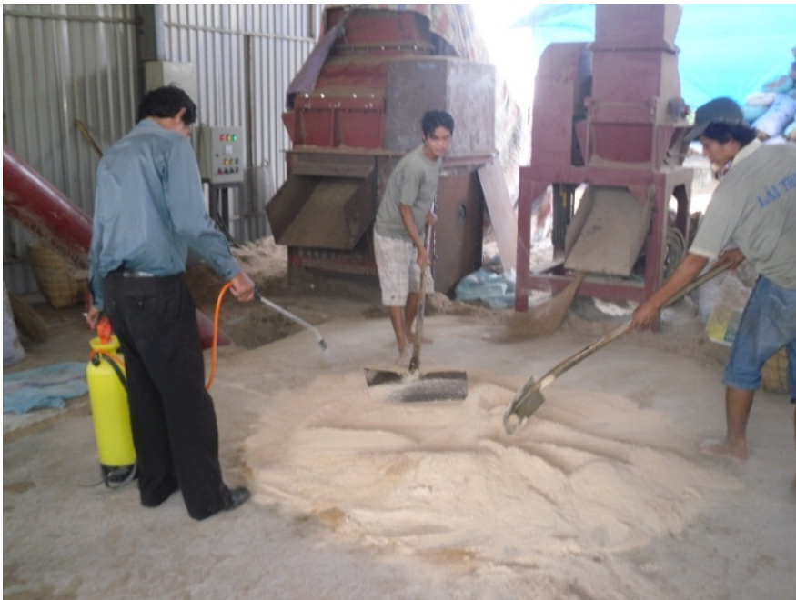
Figure 49. Increasing moisture to ground rice husks (Photo by Arvo Leinonen).
