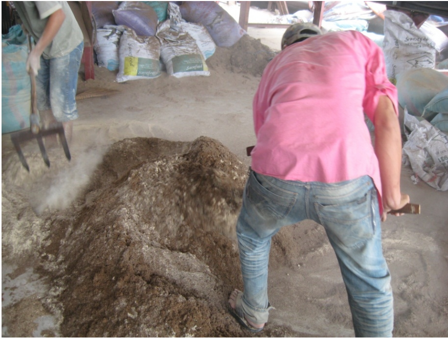
Figure 50. Blending ground bagasse and rice husks (Photo by Duc Vu).
