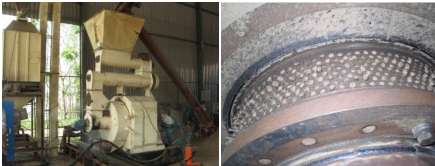
Figure 46. Pellet press, screw, belt and bucket conveyors and intermediate pellet hopper in pellet production line (left) and ring die of the pellet machine (right) (Photos by Duc Vu).
