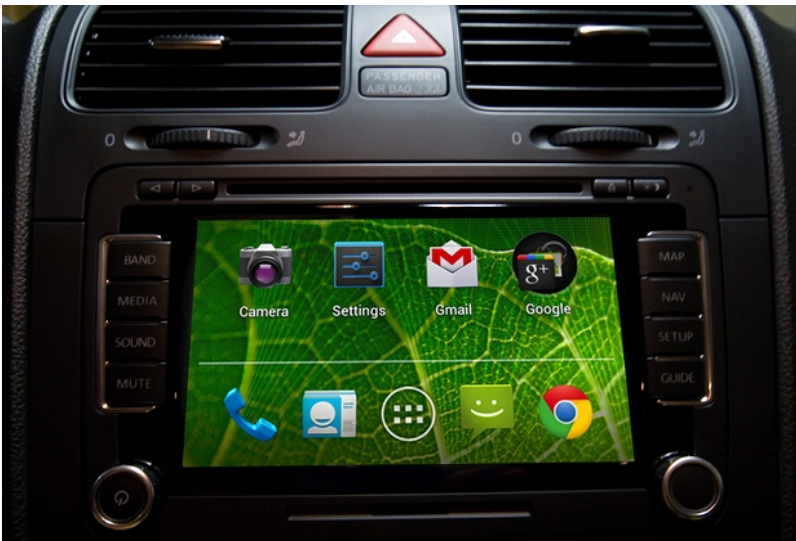
Figure D9. Android mobile phone display on an IVI screen (courtesy of ZDNet).
