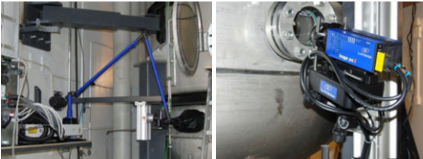
Figure 1. Laser (left) and camera (right) of the PIV system.
