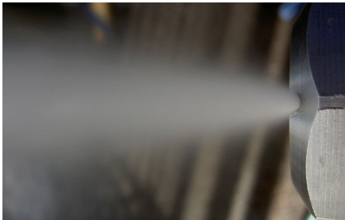
Figure 7.17. Atomization test on-going at the Oilon laboratory in Lahti (Oilon 2013).
