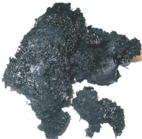
Figure 9.2. Coking in the supply line due to overheating of bio-oil (Preto et al. 2012).
