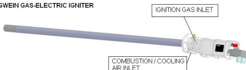
Figure 7.22. High quality gas-electric igniter can also be used as pilot burner if needed.
