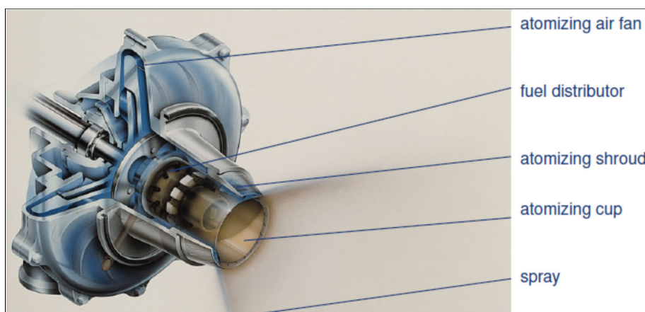
Figure 7.4. The SAACKE rotary cup atomizer.
