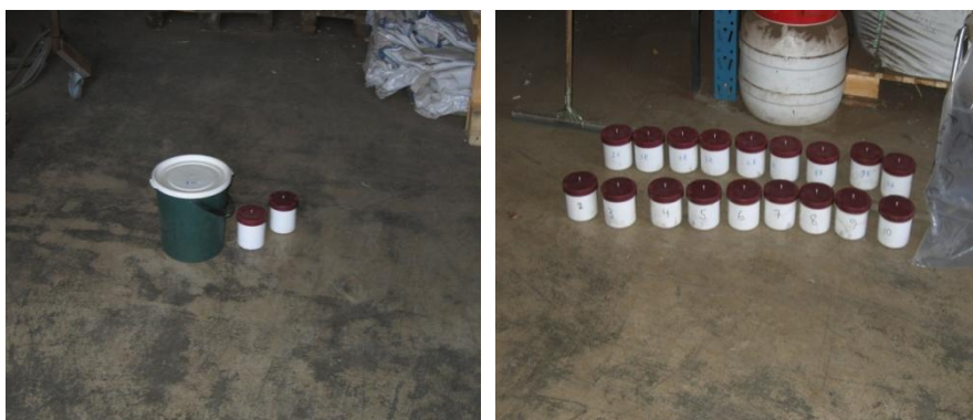
Figure 29. Increment sample division (left) into two MR analysis samples and one truck load’s increments (10) in MR analysis pots (right).
