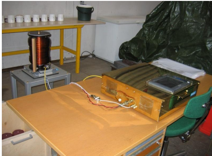
Figure 16. Vaisala MR moisture gauging device (CPU in front and electromagnet on the left; behind and near the wall are sample pots, which will be put into the magnet for the measurement.).
