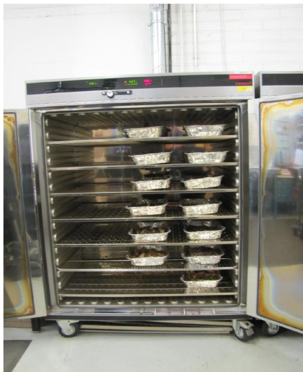
Figure 17. Typical sample drying oven and sample containers.
