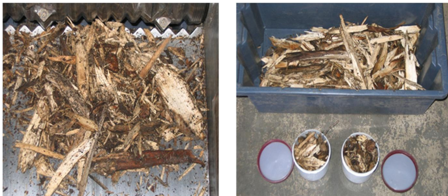
Figure 4. Stump sample particle size reduction and division for moisture content measurement using the MR device.
