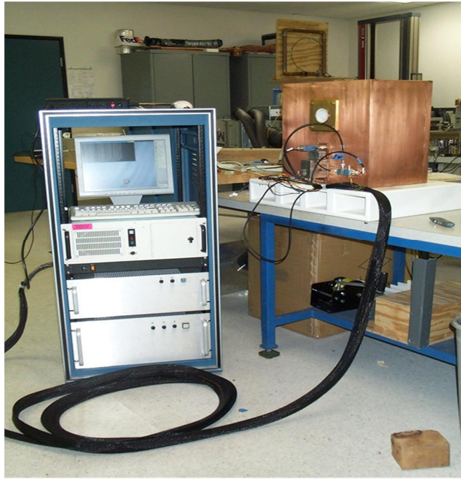
Figure 15. Light MR device (on the table: magnet, RF coil, amplifier; on the floor: RF receiver, PC, and power supply). Cable length between magnet and CPU: 6 m (Magnuson 2004).
