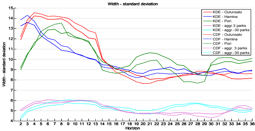
Figure 23. Standard deviation of 90% probability interval. Aggregated forecast do not have as variable uncertainty interval widths for different weather situation than the single turbine sites.
