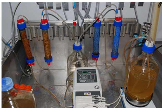
Figure 8. Experimental set-up of fixed bed bioreactors.
