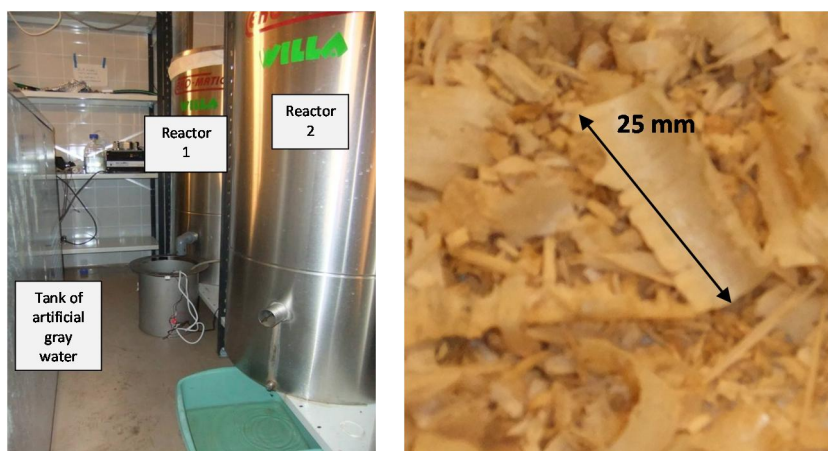
Figure 10. a) Experimental set-up of FBBR system consisted of a tank of artificial grey water, two cylindrical reactors, and pumps. b) Wood chips served as carrier material in FBBR system.
