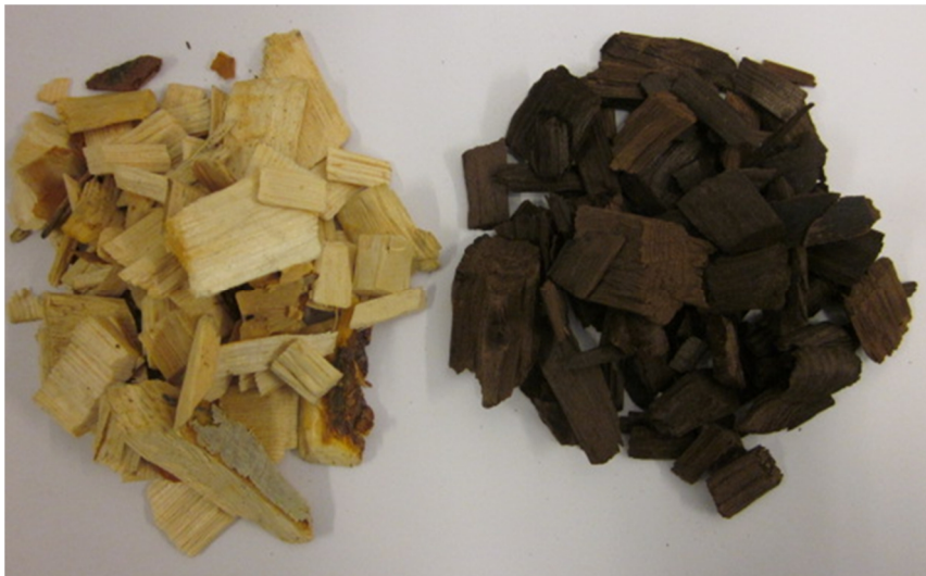
Figure 25. Wood chips and torrefied wood chips used in the fixed-bed gasification tests.
