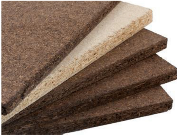
Figure 29. Samples of particle boards produced from spruce chips and torrefied wood chips.
