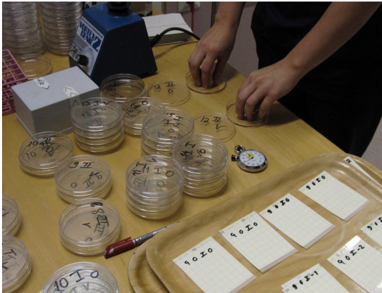
Figure 2. The testing was performed using a modification of the standard EN1500 i.e. without using artificial inoculation. Microbes from fingertips were transferred to dilution solution and cultured on 3M™ Petrifilm™ Aerobic Count Plates. The results from fingers before and after disinfection showed that the testing with the manual dispensers gave a reduction of up to 0.7 log-units and with the Kiilto Non-Touch device up to 1.1 log-units.
