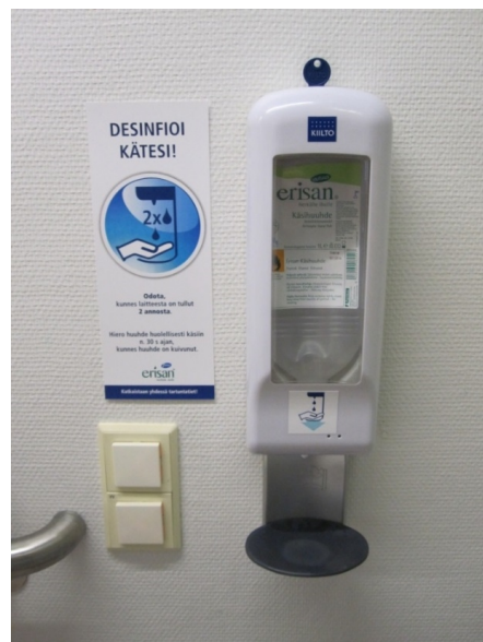
Figure 1. The dosing of the disinfectant with the Kiilto Non-Touch dispenser is based on impulses from the movement sensor and thus the users' hands do not touch the surfaces of the device. This dispenser is designed for use in public places, i.e. it is locked so that the disinfectant bag cannot be removed by visiting customers.
