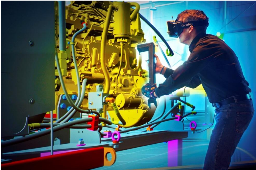
Figure 3. Using virtual prototyping for testing and analysing an assembly task.
