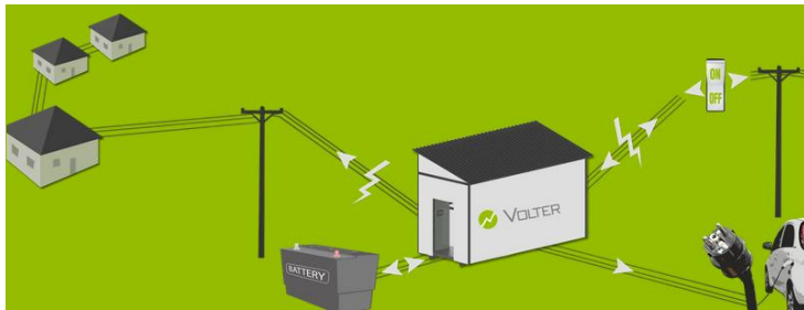
Figure 2.3. Example microgrid system marketed by Volter Oy [4].
