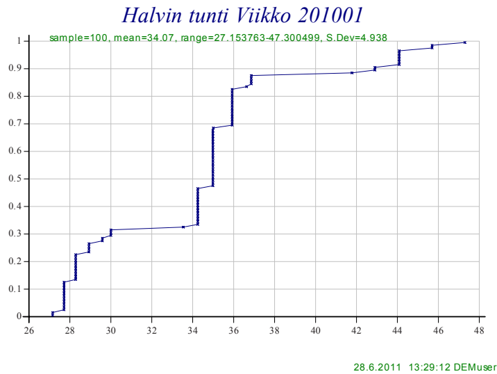
Figure A8. Probability distribution of the lowest hourly price of electricity occurring during a chosen week (first week of 2010), based on a sample of 100 simulated cases. The price of electricity is in euro/MWh on the horizontal axis, with the cumulative distribution on the vertical axis.
