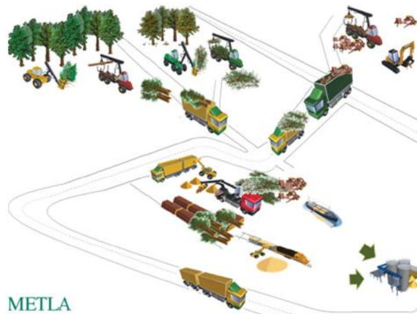
Figure 2. Forest fuel supply chain based on comminution at the terminal. (Figure: Metla)
