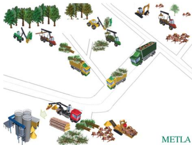
Figure 3. Forest fuel supply chain based on comminution at a power plant. (Figure: Metla)
