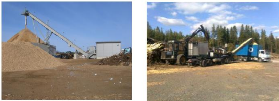
Figure 6. Examples of the space requirements of comminution machinery in a terminal. A large stationary chipper on the right and mobile chipper on the left. The mobile machinery requires significantly less space as the worksite moves along the piles being processed.
