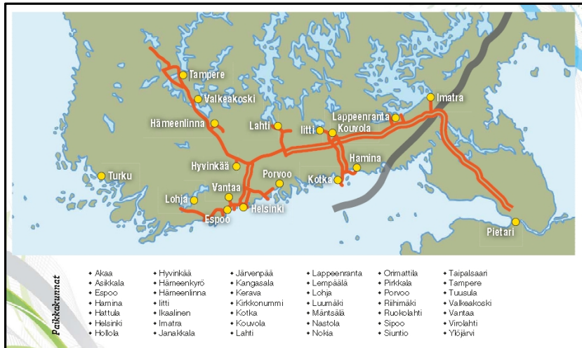
Figure 6.1.2. Finland's natural gas pipelines (Finnish Gas Association).
