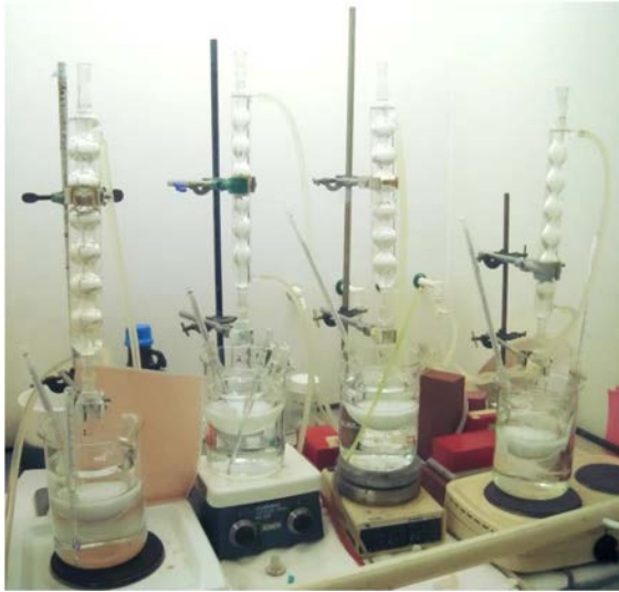
Figure 4. Test setup of the chemical effect tests.
