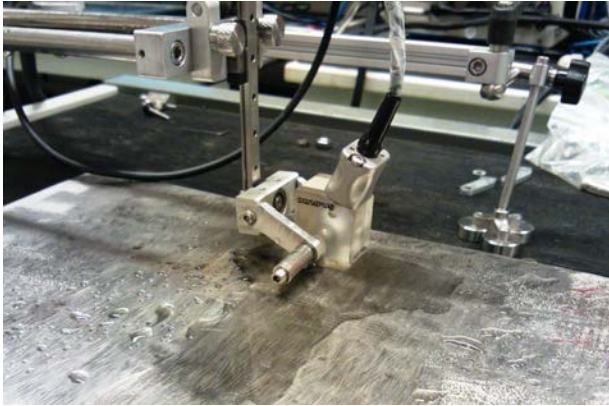
Figure 1. Scanning of the test plate with phased array ultrasonic technique.
