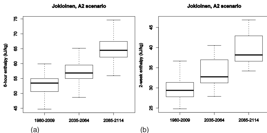
Figure 4. The box-and-whisker plots of annual maximum (a) 6-hour and (b) 2-week enthalpies at Jokioinen based on observations in 1980-2009 (left), and around the years 2050 (middle) and 2100 (right), based on model projections under the A2 scenario. Shown are the lowest maximum, the 25 th , 50 th and 75 th percentiles, and the highest maximum. Note the different vertical scales.
