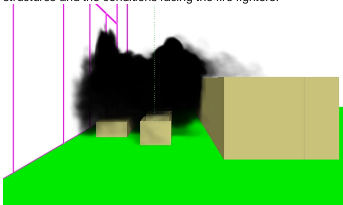
Figure 2. Smoke plume from transformer fire when 10 m/s wind is blowing from the direction of the turbine hall towards the diesel building.
