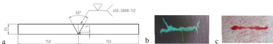
Figure 1. a) Schematic picture of the sample and liquid penetrant indications of b) thermal fatigue crack and c) mechanical fatigue crack.
