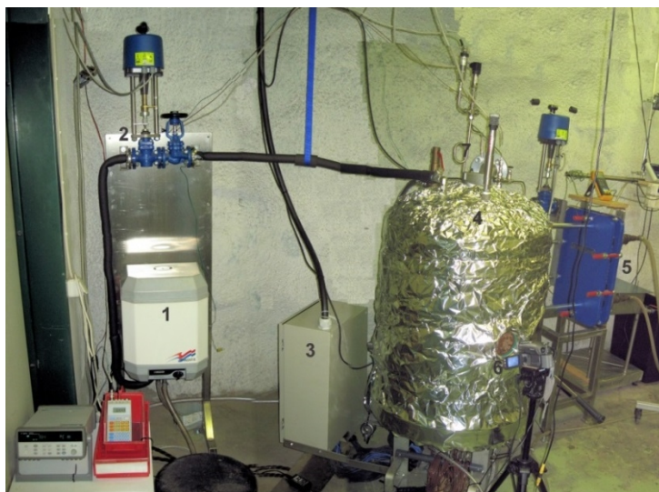
Figure 2. The COOLOCE test facility. (1) feed water pre-heater, (2) feed water control valve, (3) connection box (power input), (4) pressure vessel, condenser and scale (steam removal), (6) video monitoring, (7) pressure gauges.
