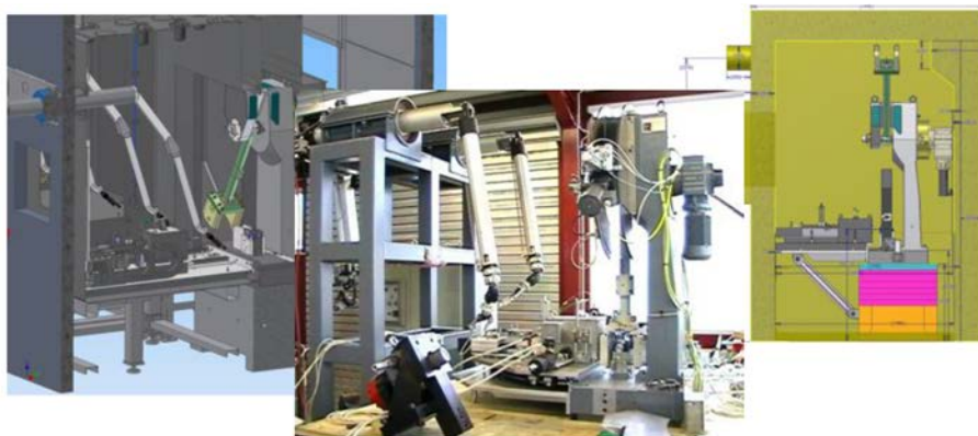
Figure 2: Examples of different hot cell installations showing space requirements for hammer, tempering unit and manipulators.
