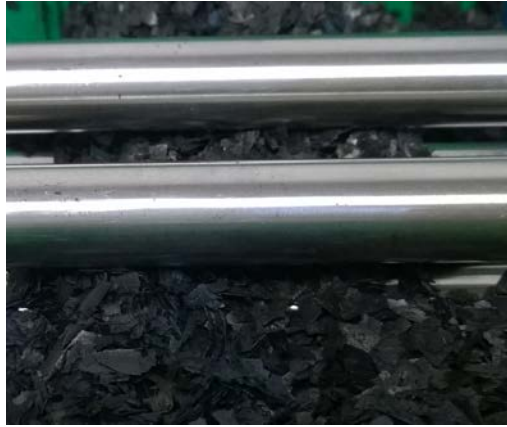
Figure 3. A part of steam generator tubing in a mock up. The two lowest tubes are submerged into the black magnetite pile.
