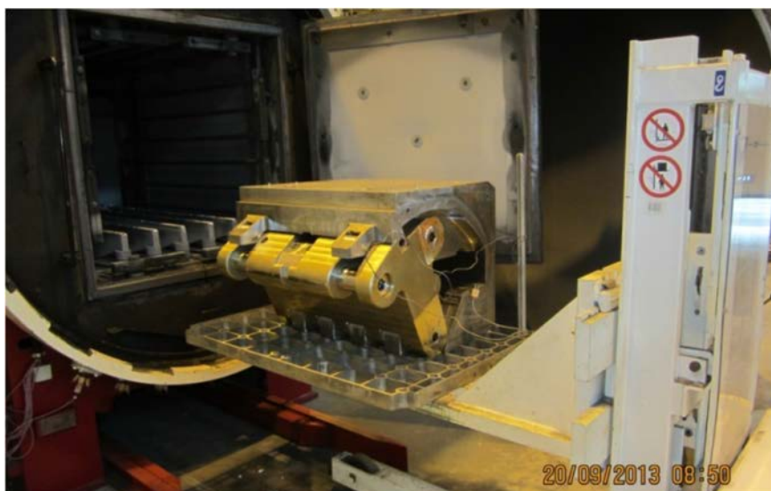
Figure 2.8. Cassette locking system after heat treatment in a vacuum furnace.
