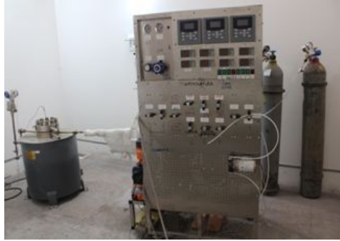
Figure 3. Test equipment for stress corrosion cracking with U-bend specimens
