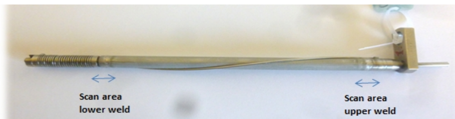
Figure 7. Image of one of the fuel pin mock-ups, CT scan area and weld position.
