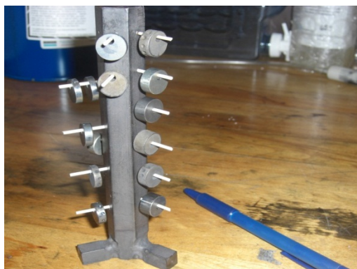
Figure 3. The samples were hung from the alumina arms of a customized 316 stainless steel tree before being placed into the SCW autoclave.
