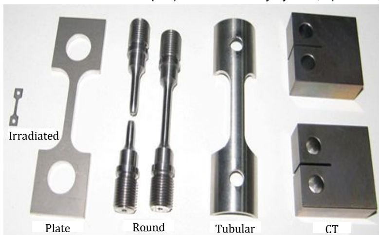
Figure 3. Types of specimen for SCC tests
