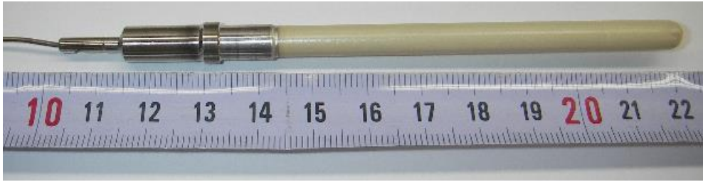
Figure 3: Picture of a reference electrode for use in SCW.
