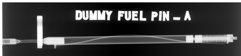
Figure 10. Radiographic 2D X-Ray image of the fuel rod mock-up 1 taken after the depressurization test.
