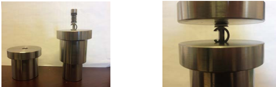
Figure 2: Picture of upper and lower platens and c-ring installation for Instron validation experiment.
