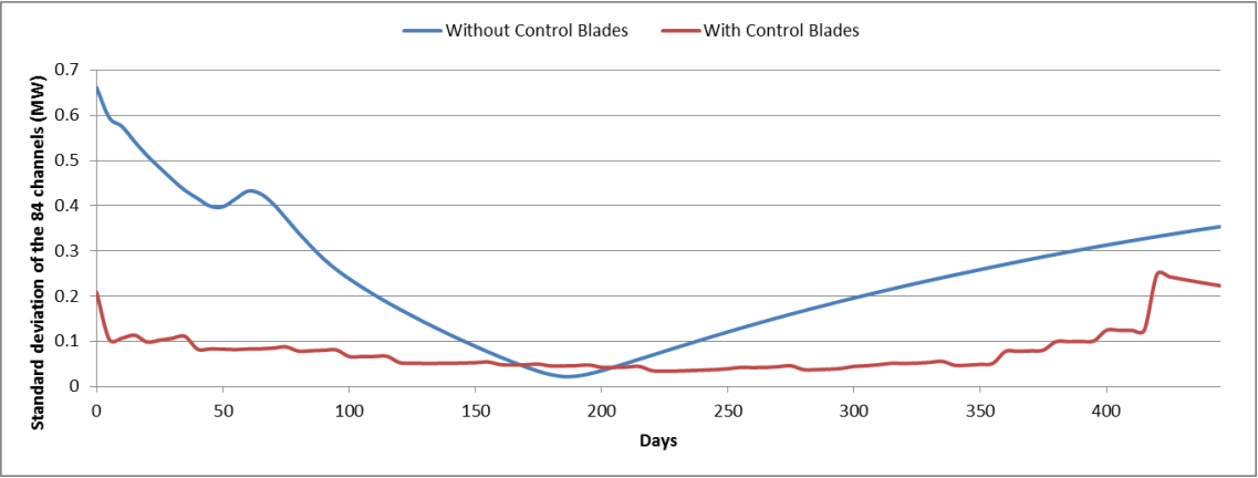
Figure 12. Standard deviation of the 84 channel powers throughout the cycle, with respect to their individual power target
