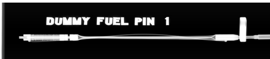
Figure 13. Radiographic 2D X-Ray image of the fuel rod mock-up 2 taken after completing Test 2A.
