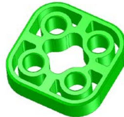
Figure 5. Spacer (support) of the fuel assembly.
