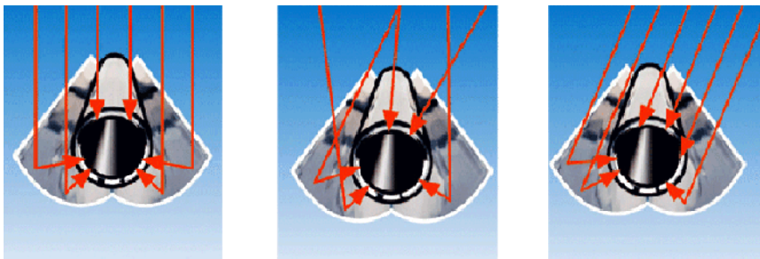
Figure 15. Evacuated tube solar collector with parabolic reflector (Kardonar, 2013).
