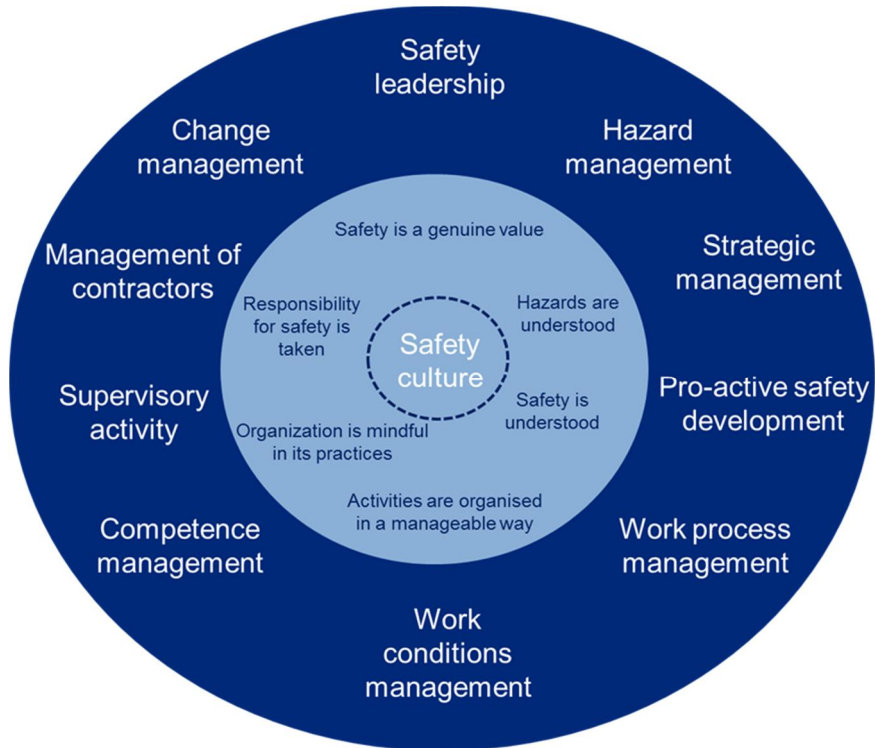
Figure 1. The DISC model summarises the criteria for good safety culture (in the inner circle) and the organisational functions that support the development of a good safety culture (outer circle) (Oedewald et al. 2011).
