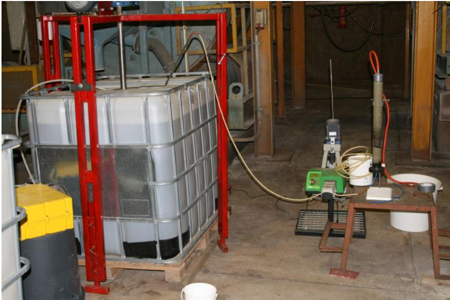
Figure 34. Test equipment of the larger column test.
