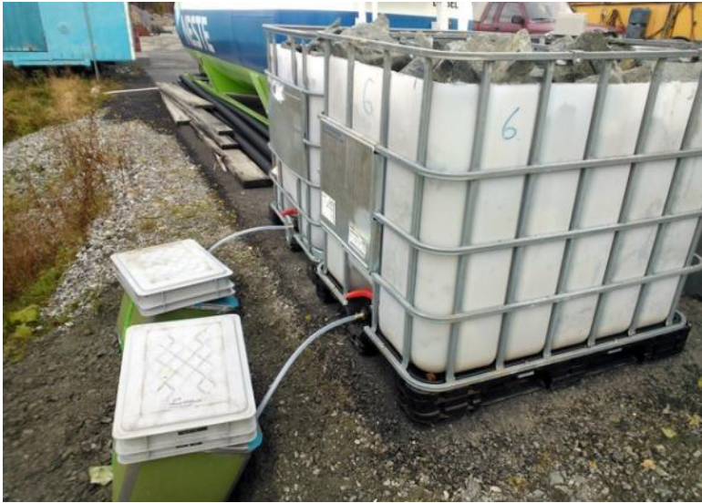
Figure 42. The aging test units 1 (front) and 2 (behind). The rain water flowing through the units was collected in the green plastic tanks below. Photo: Lauri Solismaa / GTK.
