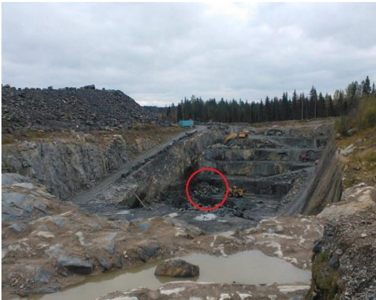
Figure 43. The material source for the test units. Left over rock material was collected immediately after the excavation of a diabase block. Photo: Lauri Solismaa / GTK.
