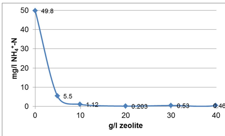
Figure 24. NH 4 + -N adsorption by clinoptilolite.
