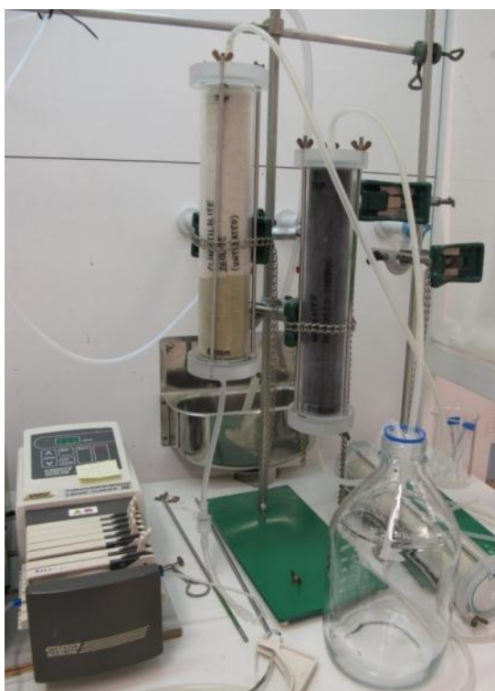
Figure 28. Second experimental setup with untreated zeolite on the left hand side (the 1st column) and untreated GAC on the right hand side (the 2nd column). The picture was taken in the beginning where the zeolite column is getting filled with water.
