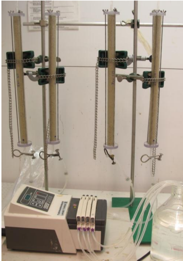
Figure 33. Four small columns. Zeolite packing was decreased before starting the experiment to facilitate flow.
