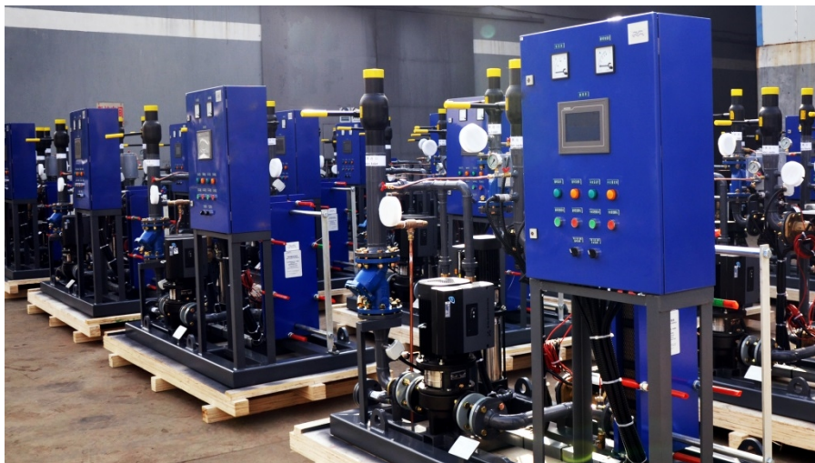
Figure 1. Building level substations (BLS) with capacity of about 10 000 m 2 each in the factory ready for shipment to Chengde, Hebei Province, China.
