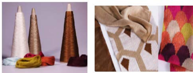
Picture 3. Lignin containing cellulose fibres manufacture with Ioncel-F process by Sixta et.al. (left) and cloths of those by Kääräinen P., Tantt M., et.al. Aalto 2014.
