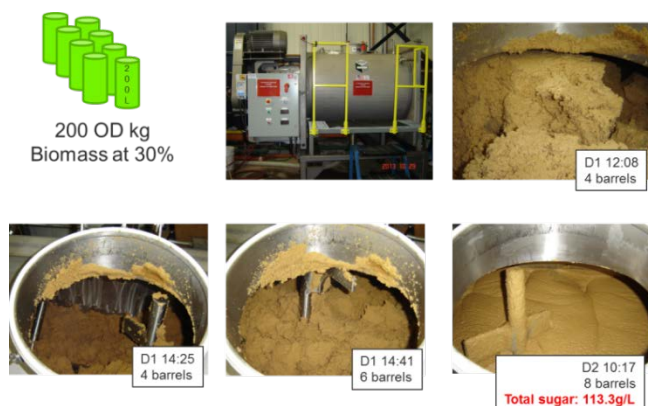
Figure 5. Fed-batch high solid enzymatic hydrolysis. Hydrolysis conditions: 20 wt % solids, 50 °C, 50 mM sodium acetate buffer at pH4.8.
