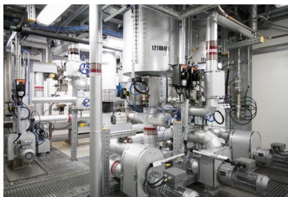
Figure 1. Digester circulation and pressurized liquor tanks in the pilot plant at Fraunhofer CBP, Leuna.
