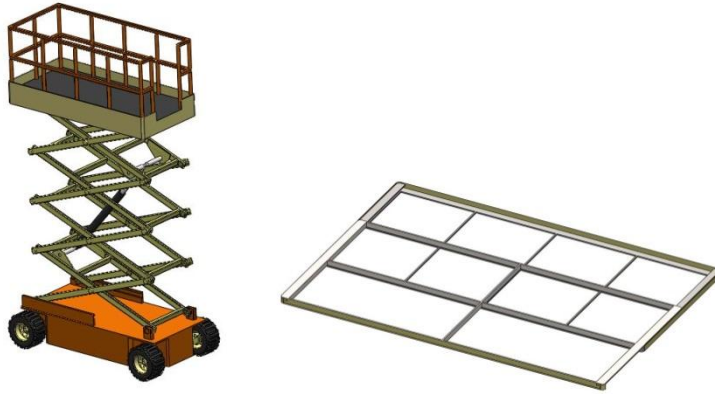
Figure 26. The original MEWP CAD model and the added y-axis module.
